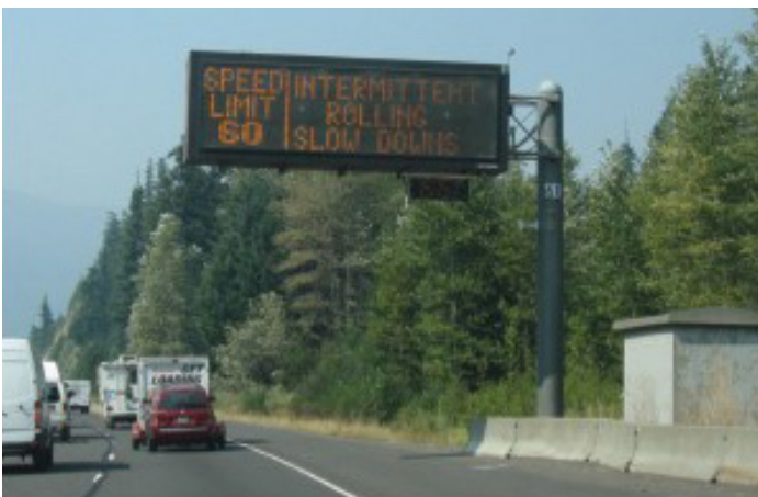
Existing permanent CMS in the area of a rolling roadblock operation can be used to supplement temporary public outreach tools during rolling roadblock operations. (Source: WSDOT)
