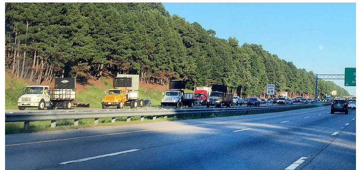
Pacing vehicles equipped with arrow or message boards and truck-mounted attenuators (TMA) safely slow and pace traffic in advance of downstream roadwork. (Source: Raleigh News & Observer)
