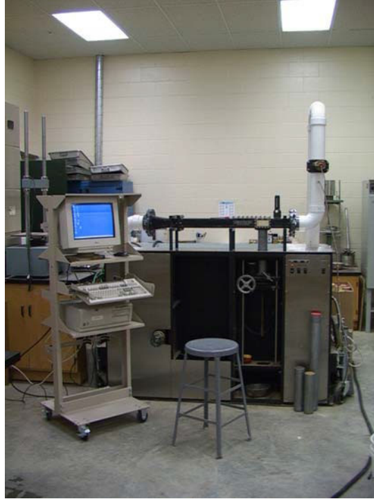
Figure 11. Minnesota Department of Transportation erosion function apparatus.
