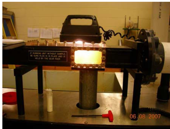
Figure 12. Water tunnel and observation window. A thin wall tube is mounted perpendicular to the water tunnel.
