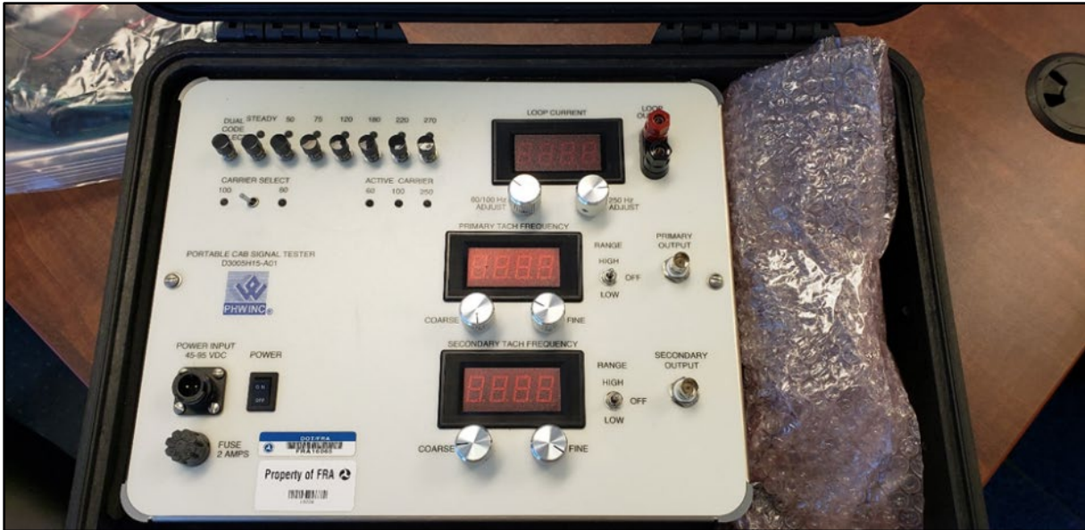
Figure H1. Image of Portable Cabs Signal Tester Utilized
