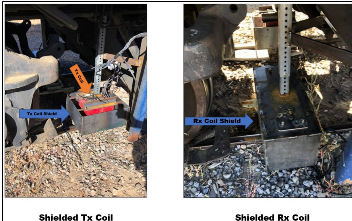
Figure 61. Images of Shielded Tx and Rx Coils
