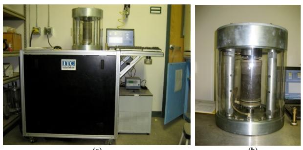
(a) (b) Figure 5: M<sub>r</sub> Specimen Assembled in SPT Machine Prior to Testing
