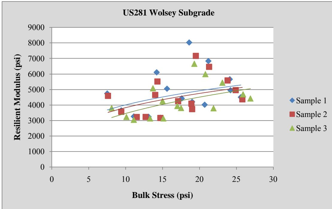
Figure 52: Resilient Modulus vs. Bulk Stress, US281 Wolsey Subgrade
