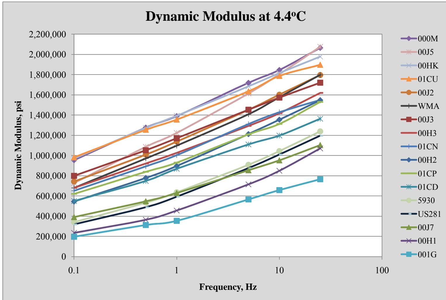
Figure 59: Dynamic Modulus vs. Frequency, 4.4°C
