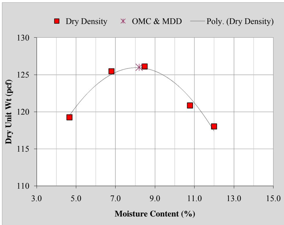
Figure 22: Dry Density vs. Moisture Content, US212 Base
