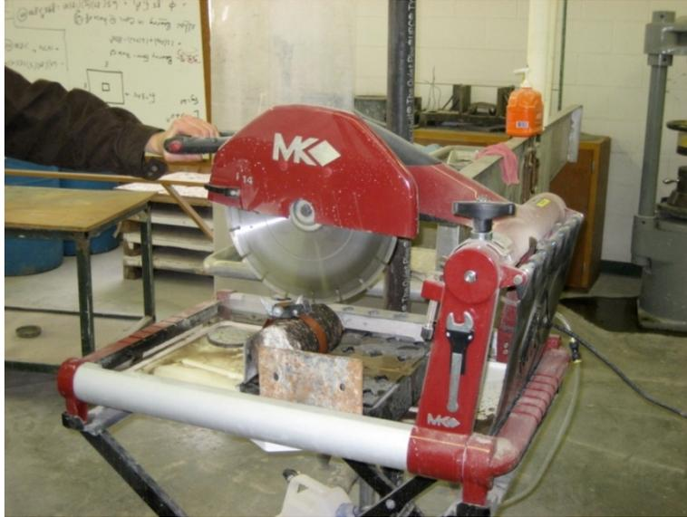
**Figure 10: Sawing HMA Sample**
