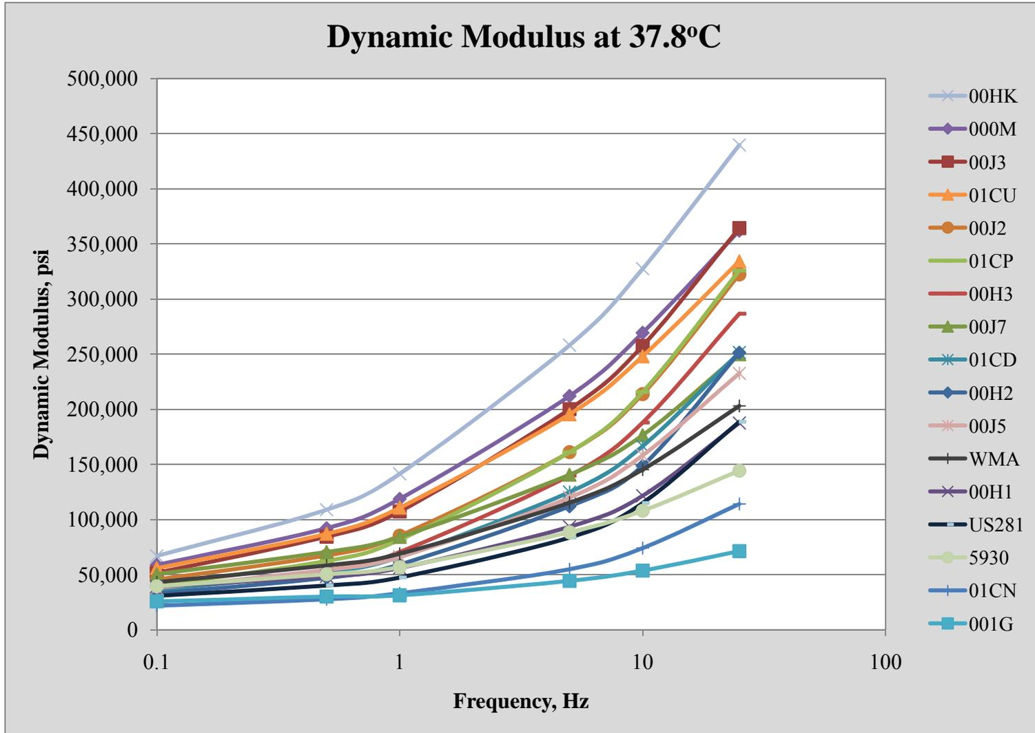
Figure 61: Dynamic Modulus vs. Frequency, 37.8°C
