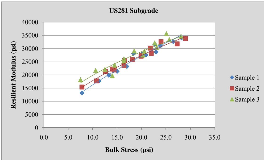
Figure 30: Resilient Modulus vs. Bulk Stress, US281 Subgrade
