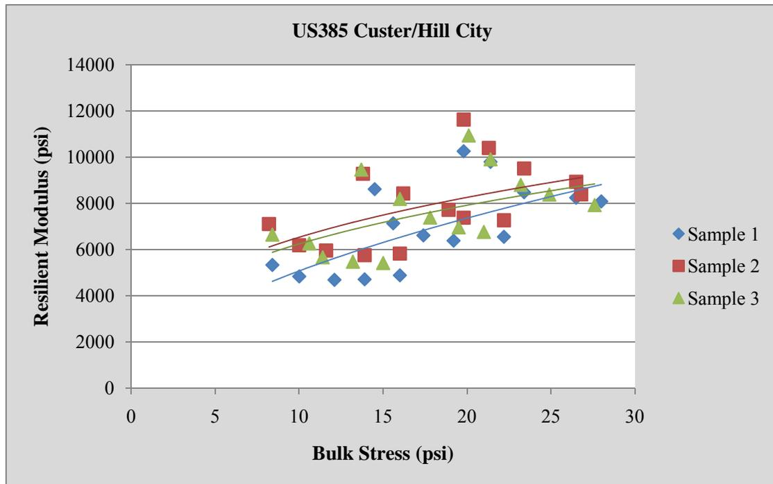
**Figure 56: Resilient Modulus vs. Bulk Stress, US385 Custer/Hill City**
