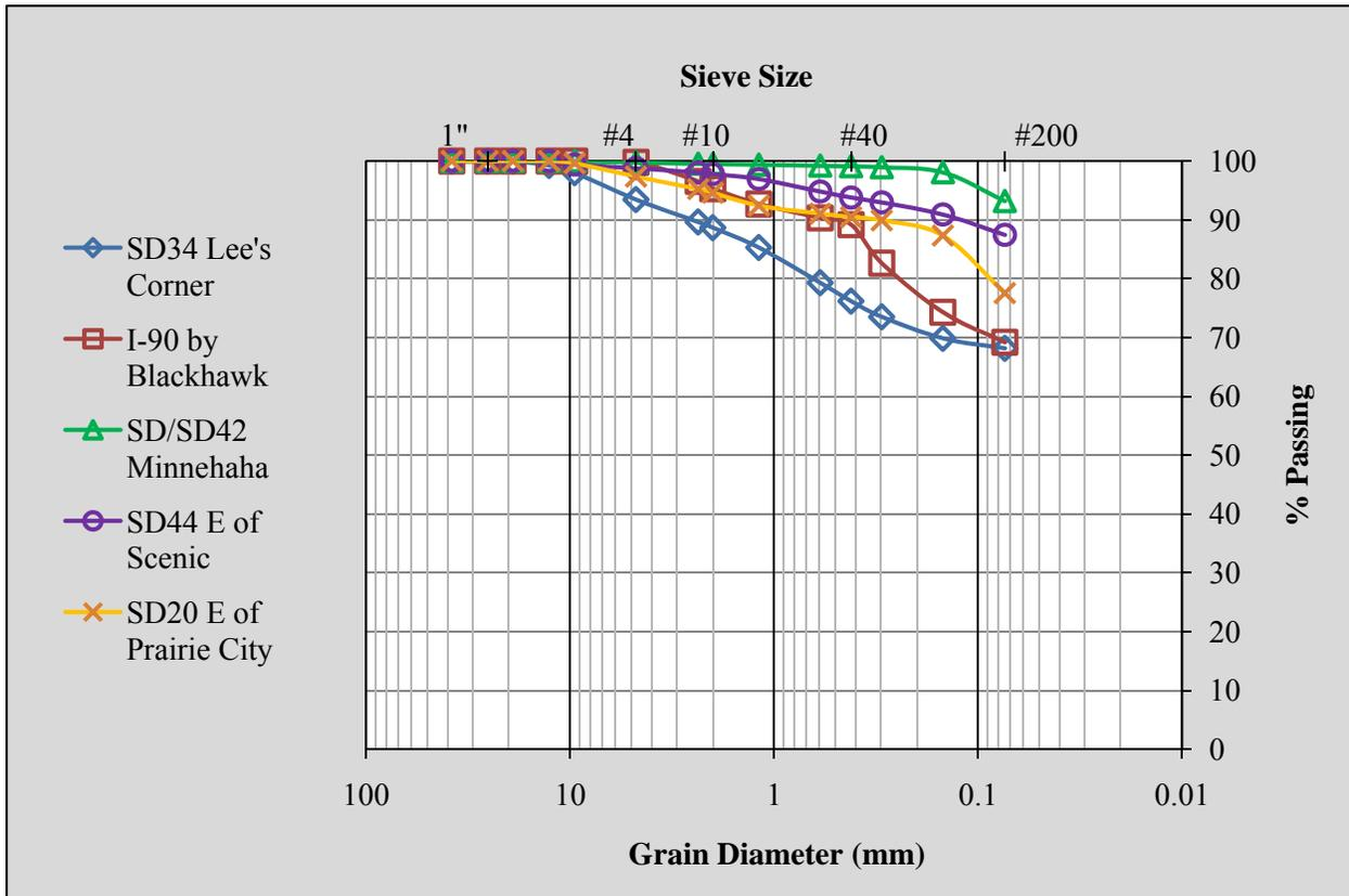
**Figure 35: Gradations for Subgrade Soils**
