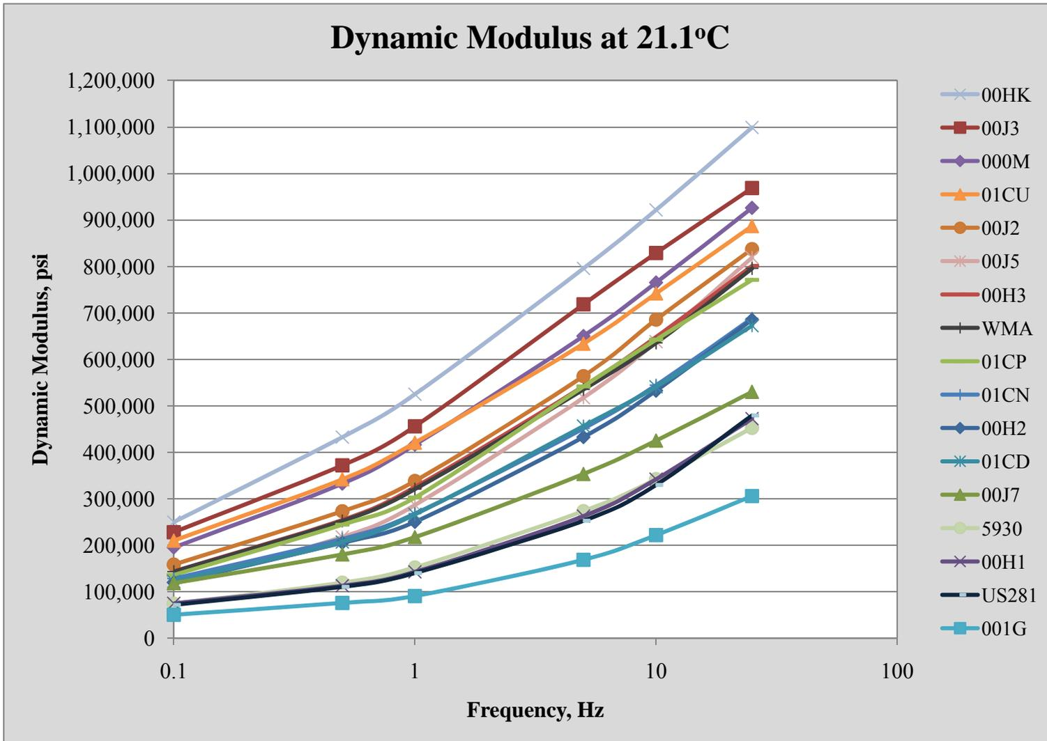
Figure 60: Dynamic Modulus vs. Frequency, 21.1°C
