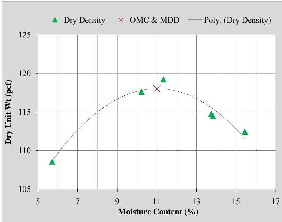
Figure 23: Dry Density vs. Moisture Content, US281 Subgrade
