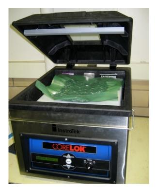
Figure 7: Maximum Theoretical Specific Gravity Sample in CoreLok Device
