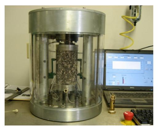
Figure 14: Dynamic Modulus Specimen Assembled in SPT Machine
