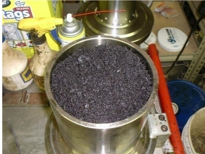
**Figure 8: HMA in Gyratory Compaction Mold**
