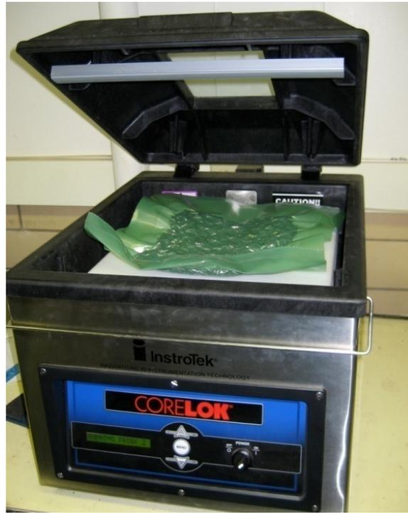
**Figure 7: Maximum Theoretical Specific Gravity Sample in CoreLok Device**
