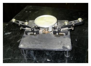
**Figure 12: Gage Point Glue Fixture**
