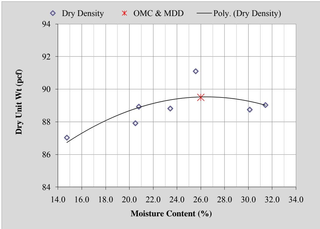
Figure 37: Dry Density vs. Moisture Content, SD34 Lee's Corner
