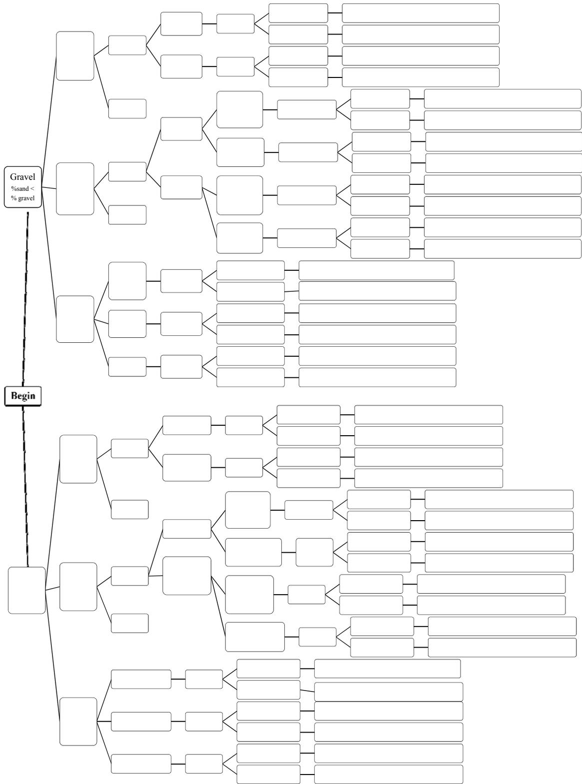
Figure 2: Unified Soil Classification System, Coarse-Grained Soils
