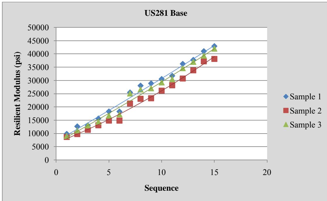
**Figure 25: Resilient Modulus vs. Sequence, US281 Base**
