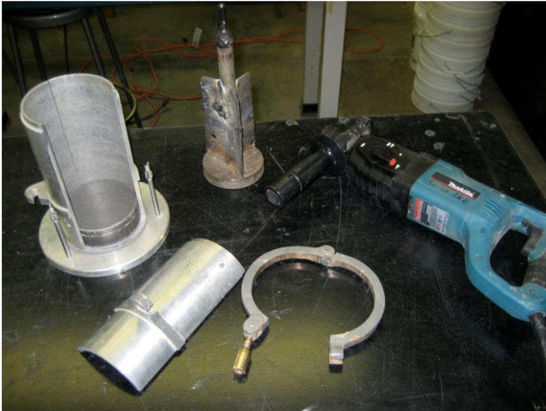
**Figure 4: Split Mold with Vibratory Compactor for Base Sample Preparation**
