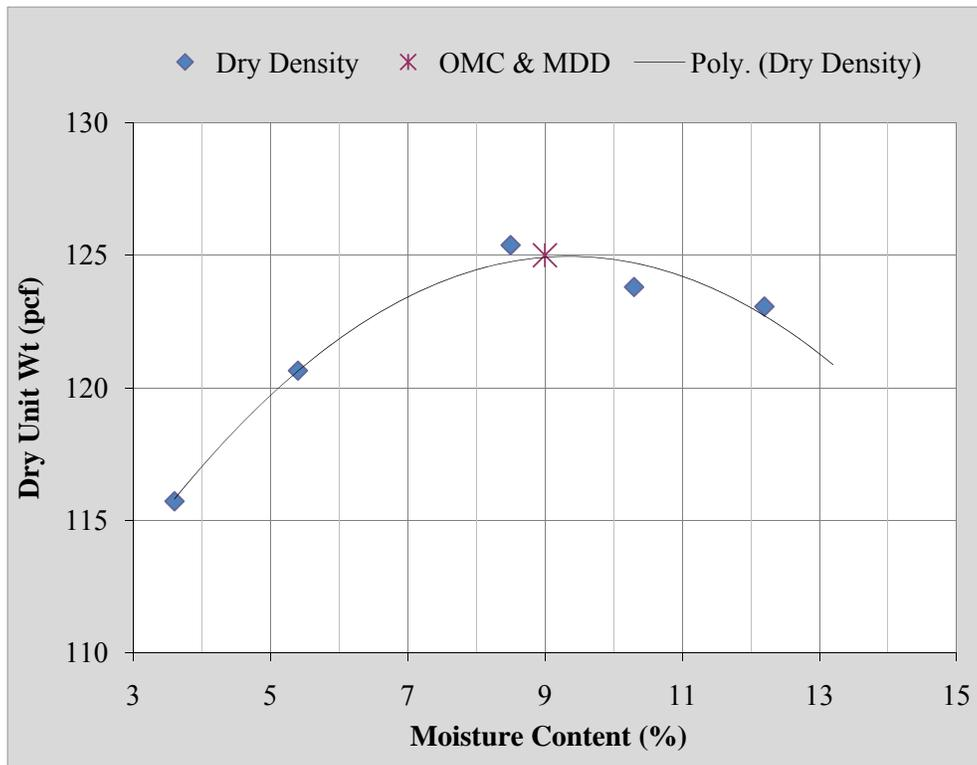
Figure 21: Dry Density vs. Moisture Content, US281 Base
