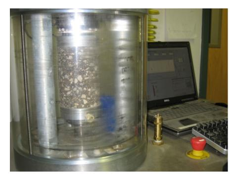
Figure 15: Repeated Load Triaxial Test Setup
