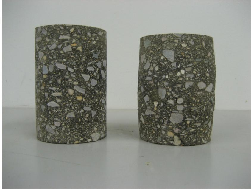
**Figure 64: Repeated Load Triaxial Samples**
