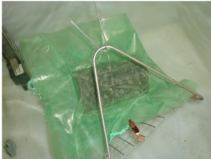
**Figure 11: Bulk Specific Gravity, Submerged Weight of HMA Sample**
