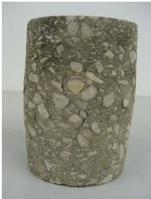
**Figure 65: Repeated Load Triaxial Sample After Testing**
