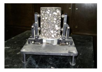
Figure 13: Gage Points Placed on HMA Sample
