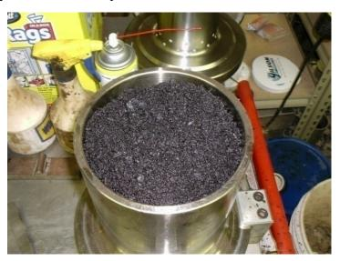
Figure 8: HMA in Gyratory Compaction Mold
