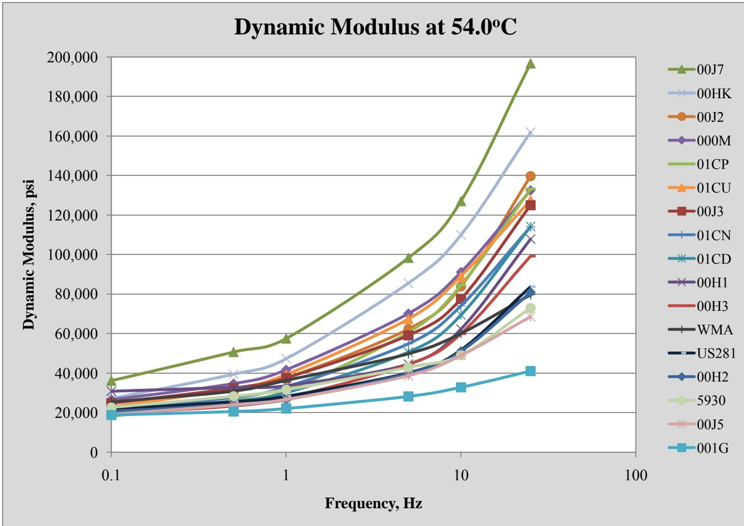
Figure 62: Dynamic Modulus vs. Frequency, 54.0°C
