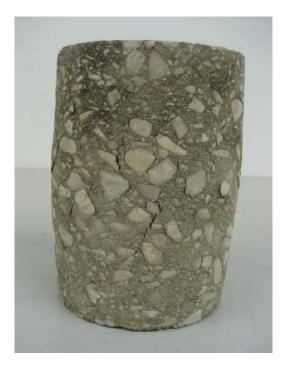
Figure 65: Repeated Load Triaxial Sample After Testing
