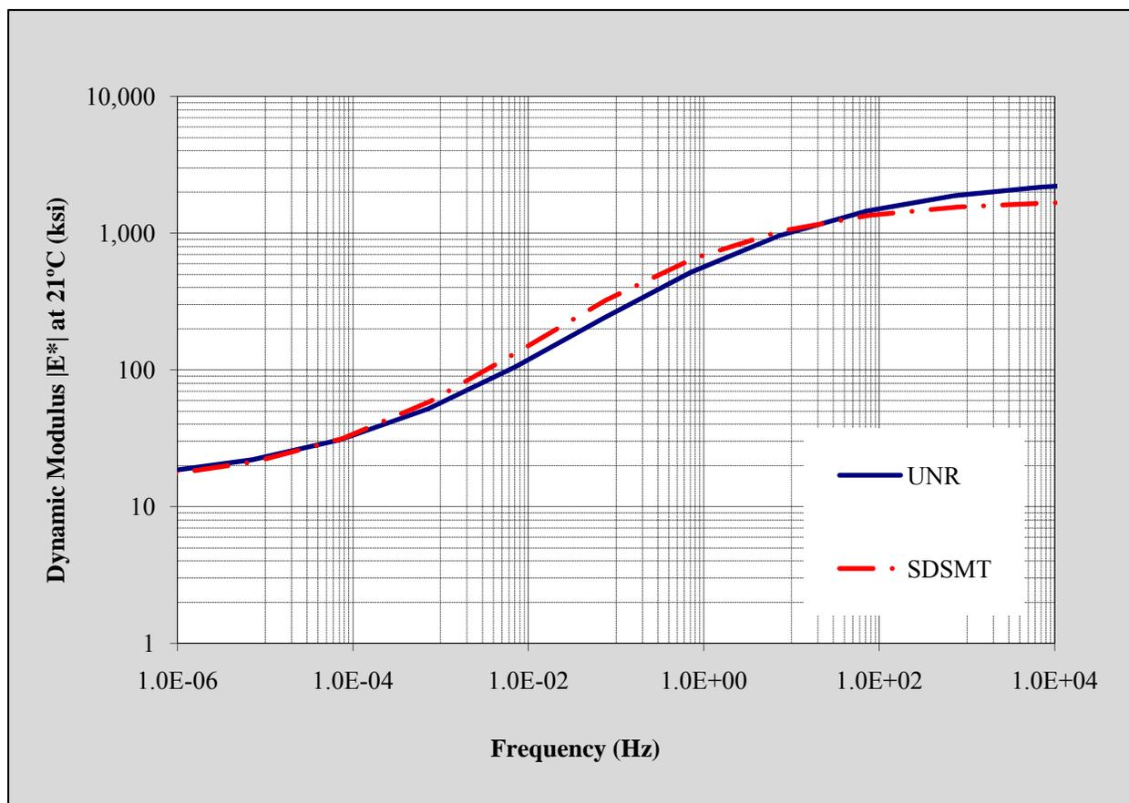
**Figure 33: US281 Master Curves for UNR and SDSM&T Data**
