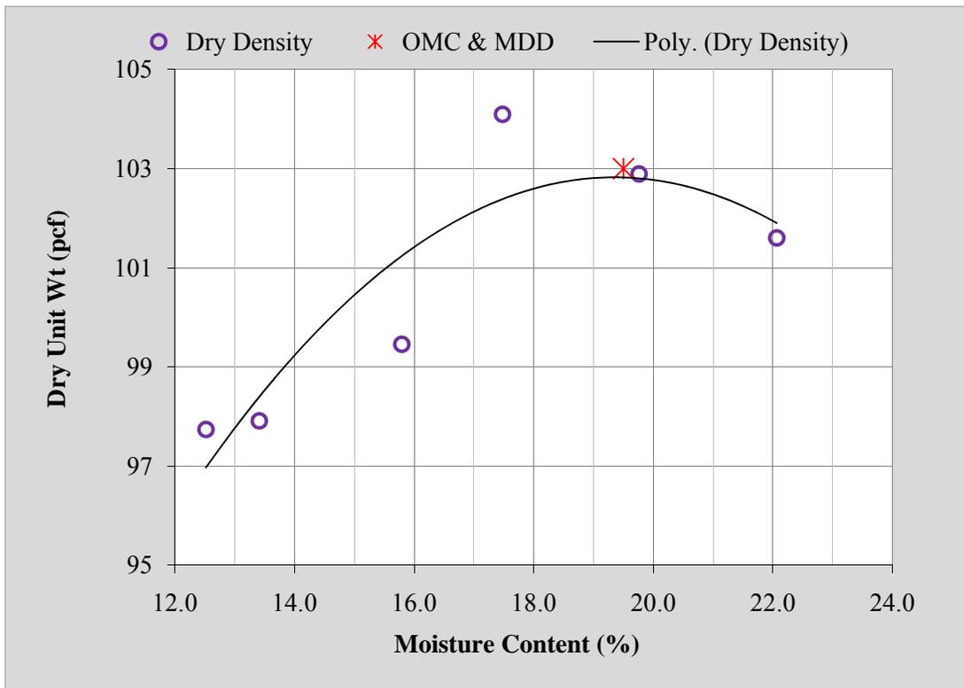
Figure 40: Dry Density vs. Moisture Content, SD44 Scenic
