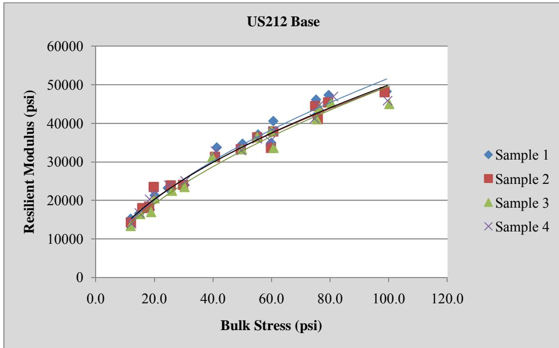
**Figure 28: Resilient Modulus vs. Bulk Stress, US212 Base**
