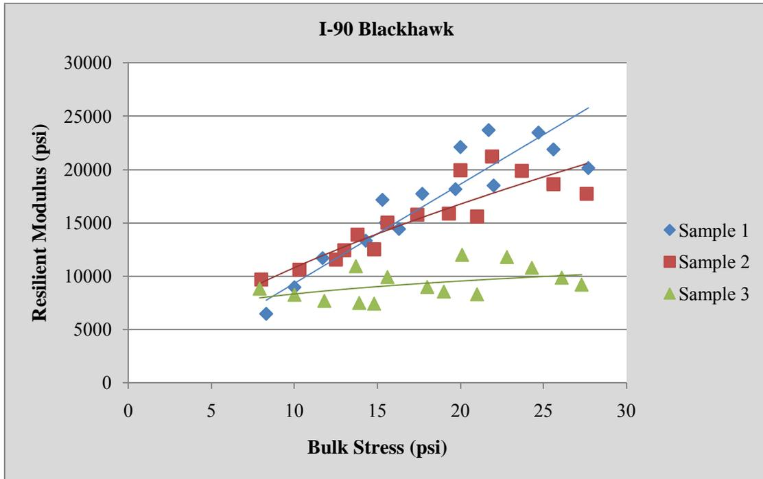
Figure 48: Resilient Modulus vs. Bulk Stress, I-90 Blackhawk
