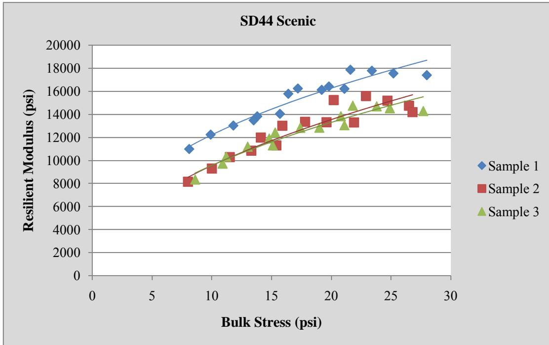
Figure 50: Resilient Modulus vs. Bulk Stress, SD44 Scenic
