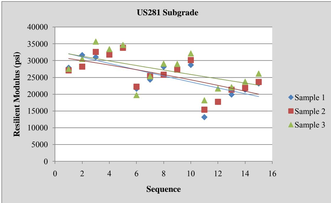
Figure 29: Resilient Modulus vs. Sequence, US281 Subgrade
