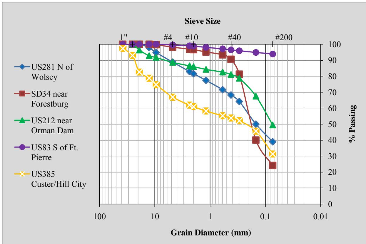
**Figure 36: Gradations for Subgrade Soils**
