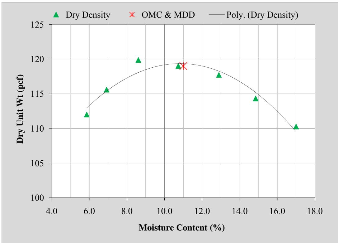
Figure 44: Dry Density vs. Moisture Content, US212 Orman Dam
