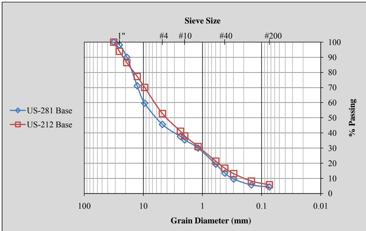
**Figure 17: Task 4 Base Material Gradations**
