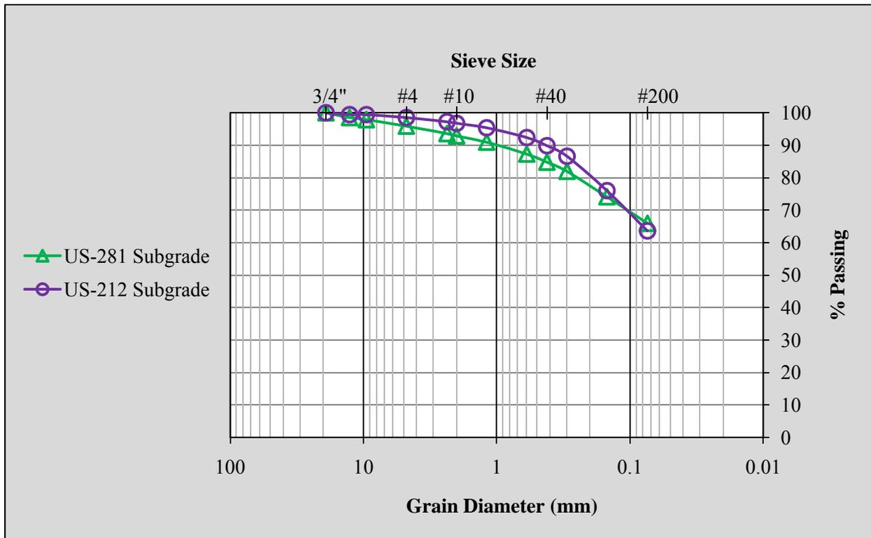
**Figure 18: Task 4 Subgrade Material Gradations**
