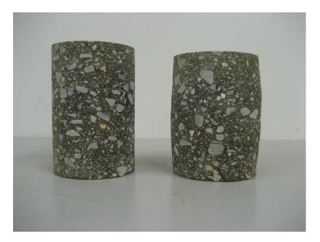
Figure 64: Repeated Load Triaxial Samples
