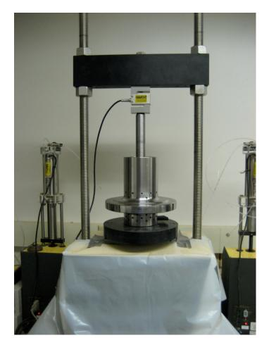
Figure 6: Assembly and Static Compactor for Subgrade Sample Preparation
