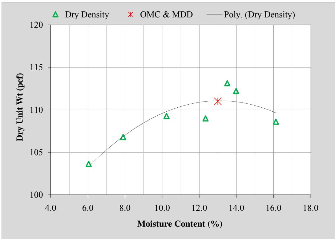
Figure 39: Dry Density vs. Moisture Content, SD11/SD42 Minnehaha County
