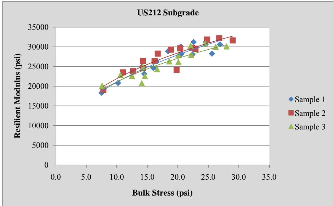
**Figure 32: Resilient Modulus vs. Bulk Stress, US212 Subgrade**
