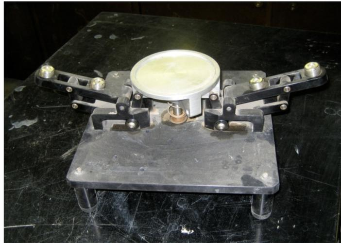
**Figure 12: Gage Point Glue Fixture**
