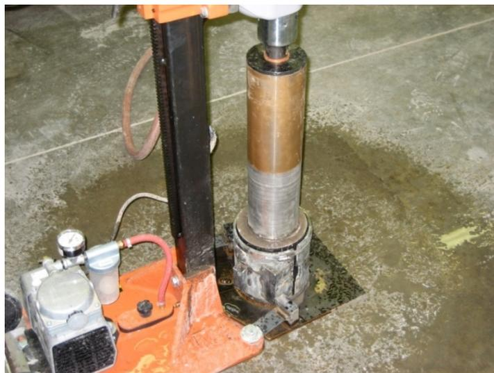
**Figure 9: HMA Coring**
