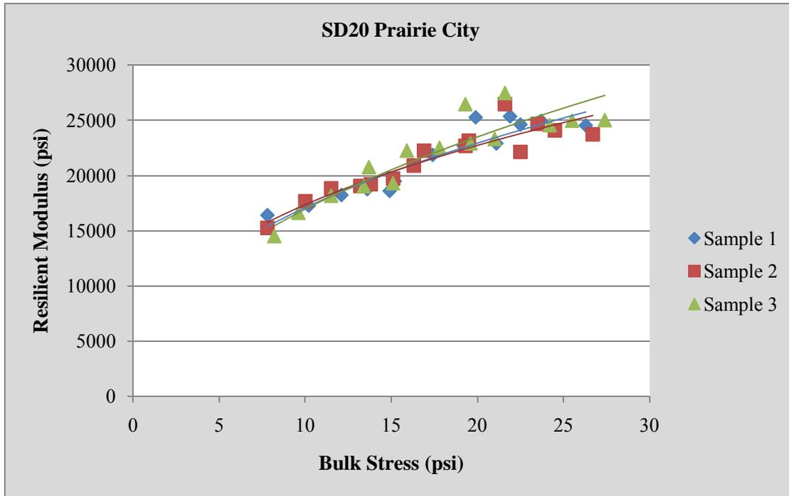
**Figure 51: Resilient Modulus vs. Bulk Stress, SD20 Prairie City**
