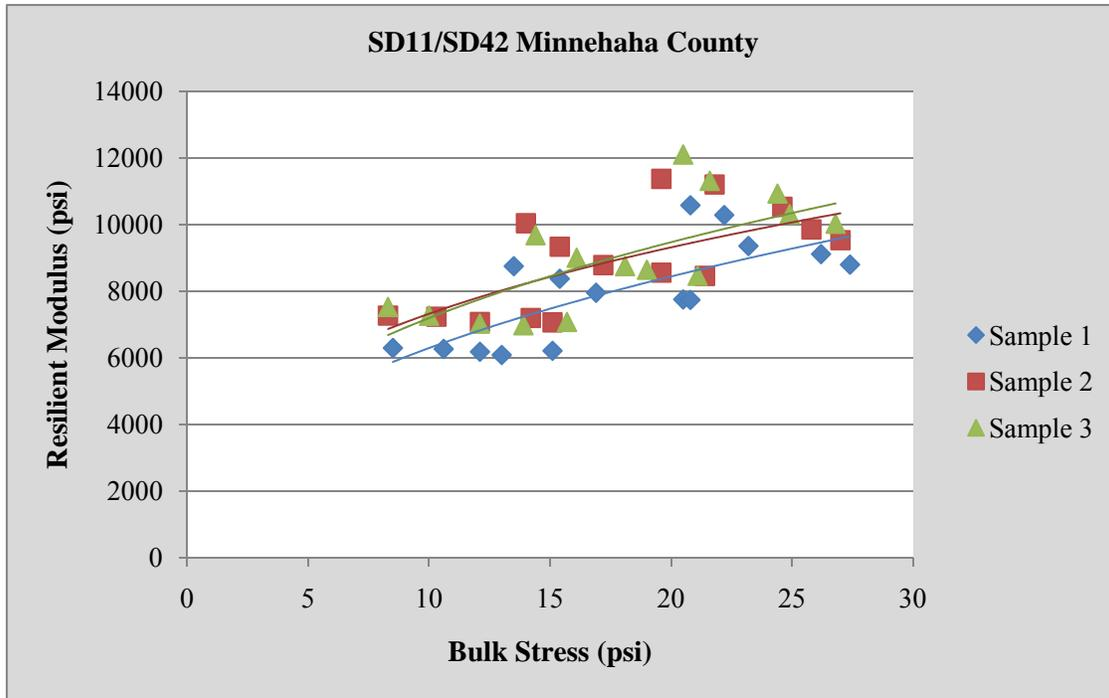
**Figure 49: Resilient Modulus vs. Bulk Stress, SD11/SD42 Minnehaha**
