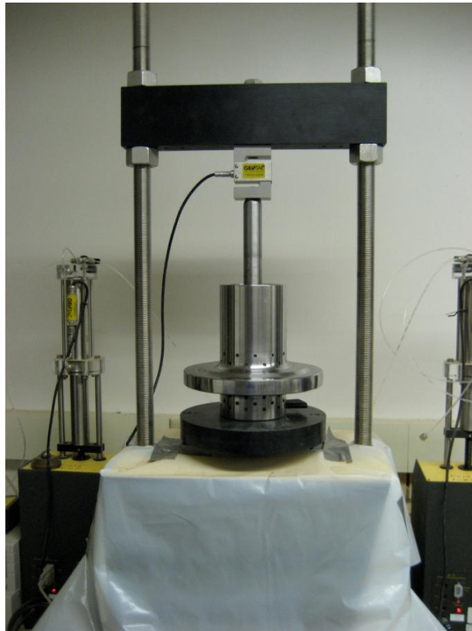
**Figure 6: Assembly and Static Compactor for Subgrade Sample Preparation**
