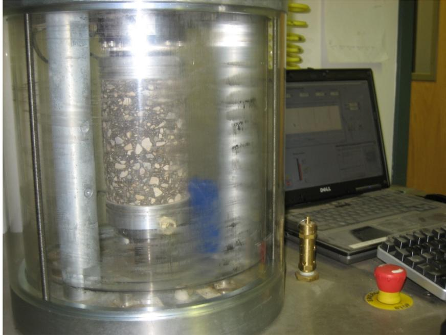
**Figure 15: Repeated Load Triaxial Test Setup**
