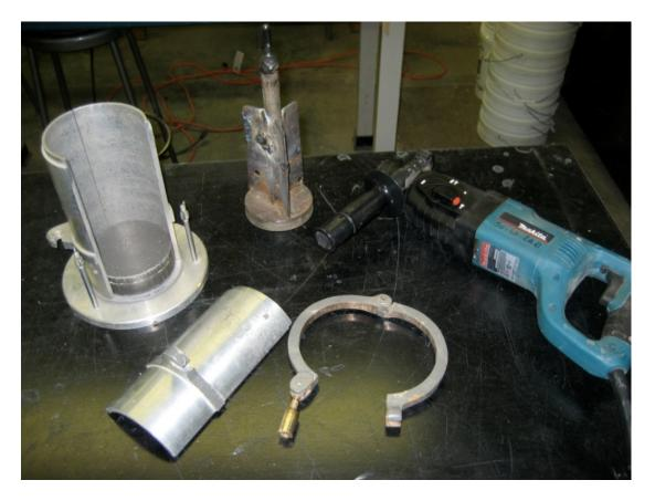
Figure 4: Split Mold with Vibratory Compactor for Base Sample Preparation
