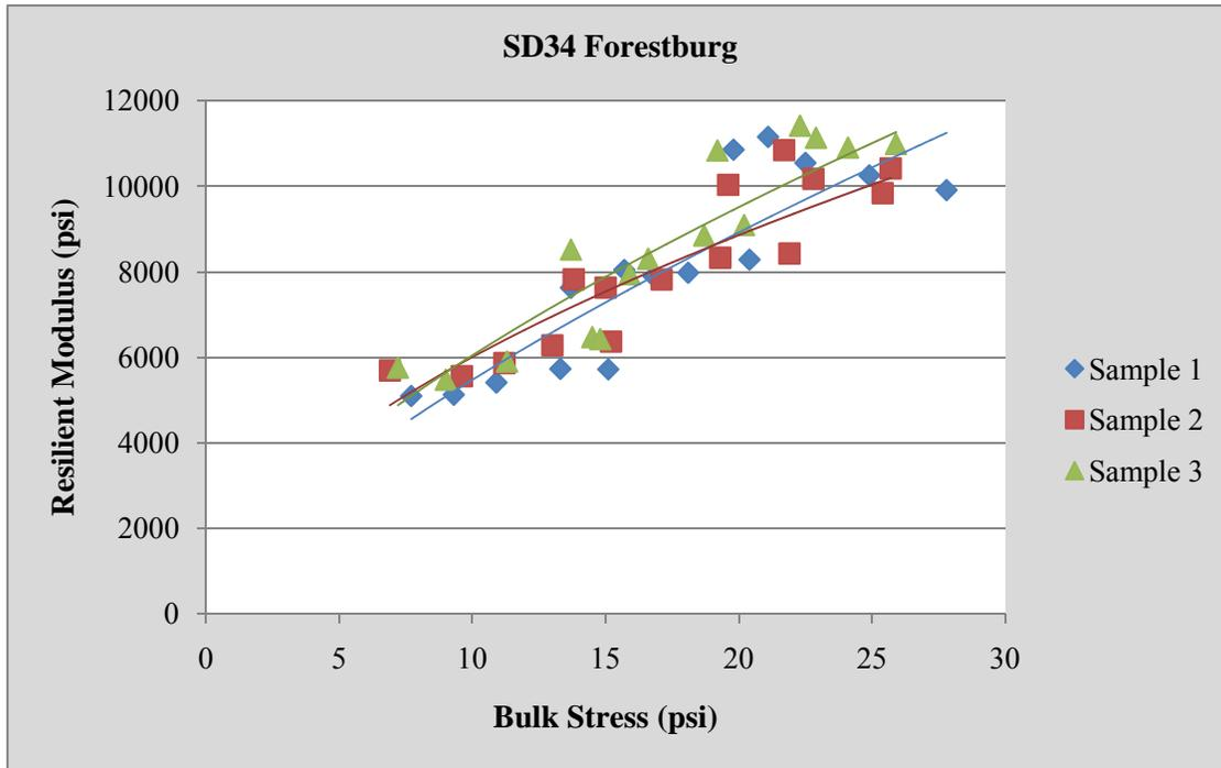
**Figure 53: Resilient Modulus vs. Bulk Stress, SD34 Forestburg**
