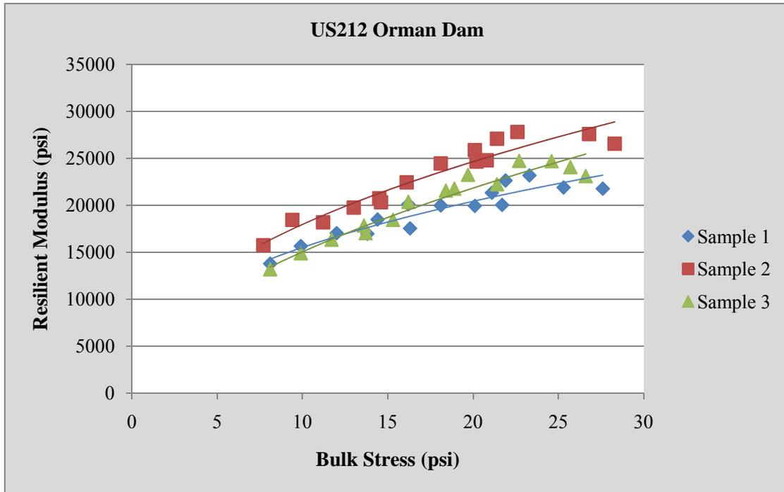
Figure 54: Resilient Modulus vs. Bulk Stress, US212 Orman Dam
