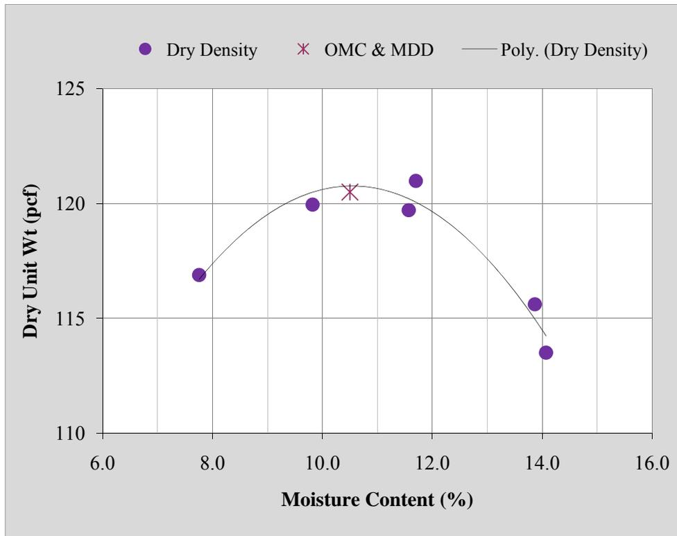
Figure 24: Dry Density vs. Moisture Content, US212 Subgrade
