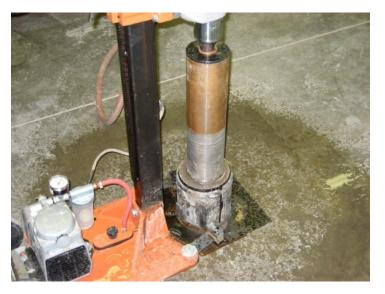
**Figure 9: HMA Coring**
