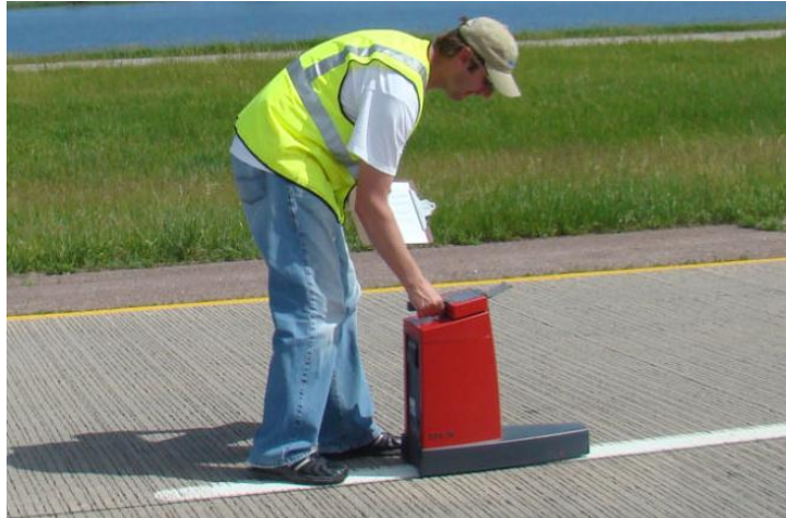
Figure 4.5: Retroreflectivity 30-Meter Geometry (Rasdorf et al., 2008)
