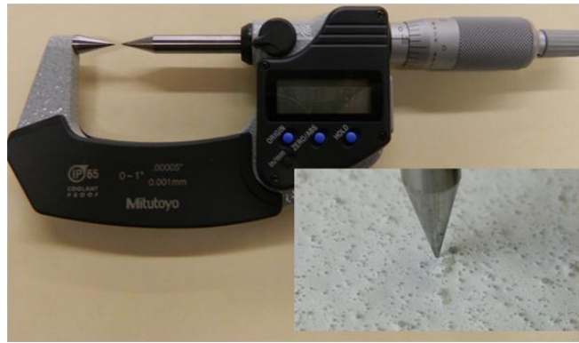
Figure 5.7: Mitutoyo 342-361 Digital Point Micrometer
