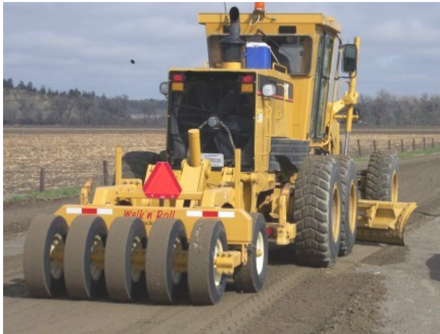
Figure 3: Walk and roller packer attached to a grader (image from http://www.walknrollpackers.com/ )
