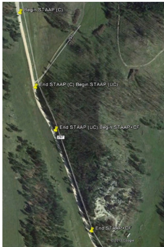
Figure 5: Layout of two STAAP and STAAP plus crusher fines sections (Google Earth images).
