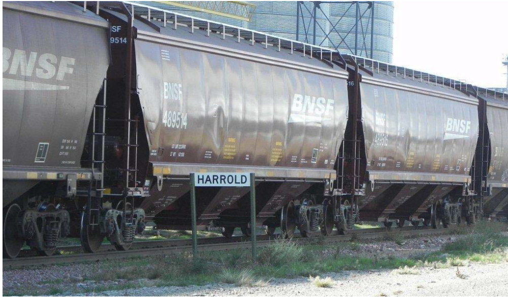
Figure 32: Minnesota, and Eastern hopper car used to carry bulk commodities able to be loaded and unloaded automatically (Courtesy of the SDDOT)
