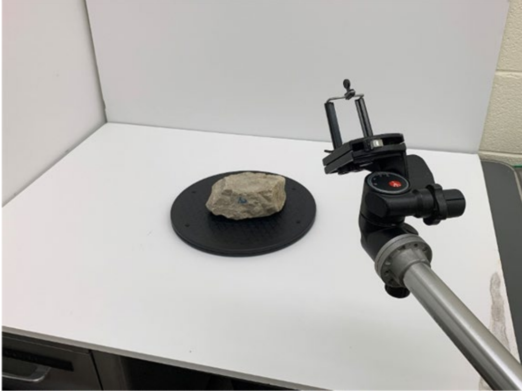
Figure 2. Photo. Equipment setup for 3D reconstruction of aggregates.
