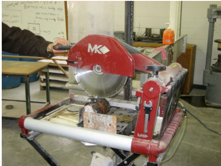
Figure 3-23: Sawing the ends of the HMA sample.
