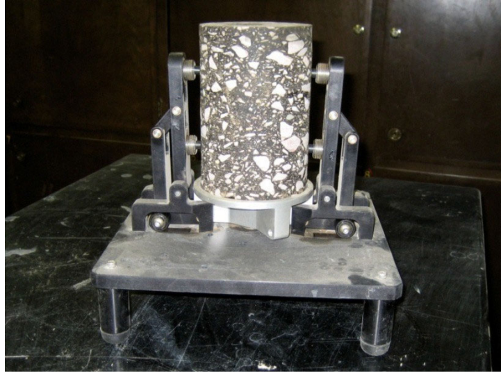
Figure 3-25: Gage points placed on HMA sample.
