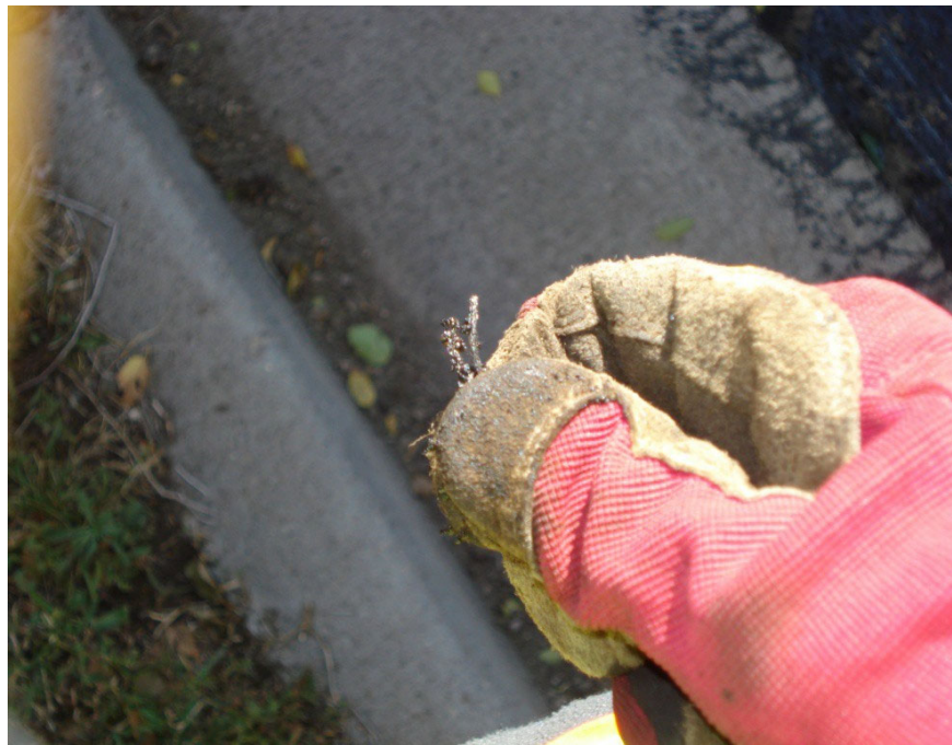
Figure 4-28: Indication of fiber clumping in Rapid City HMA mix.
