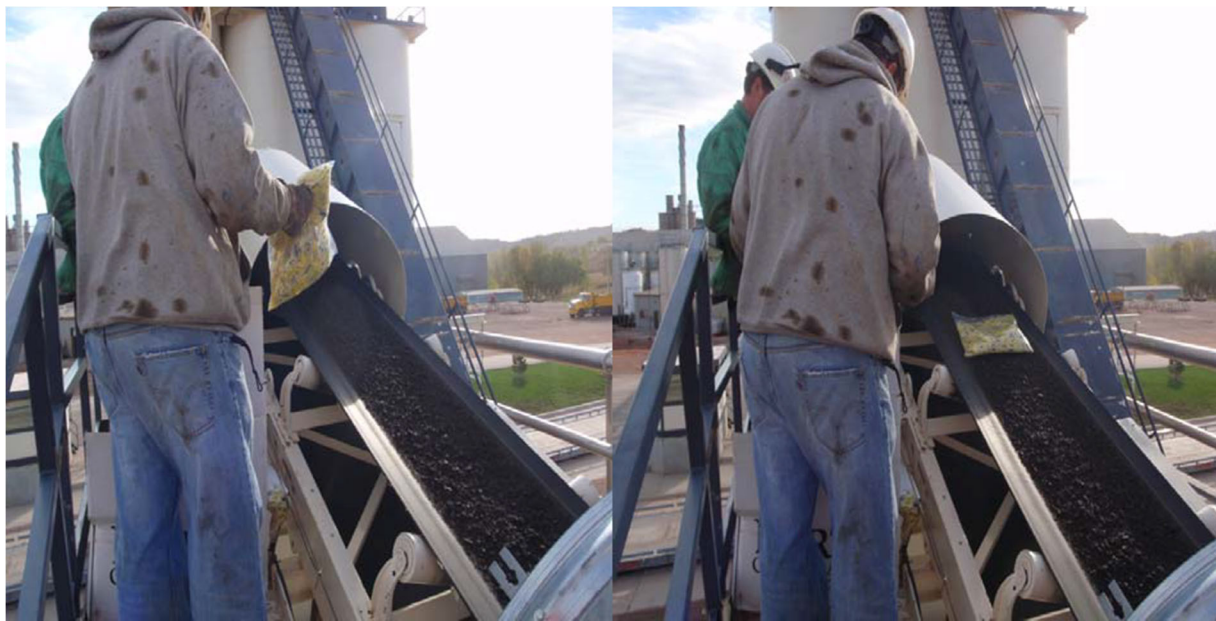
Figure 2-5: Adding the fibers onto the RAP conveyor during asphalt production.
