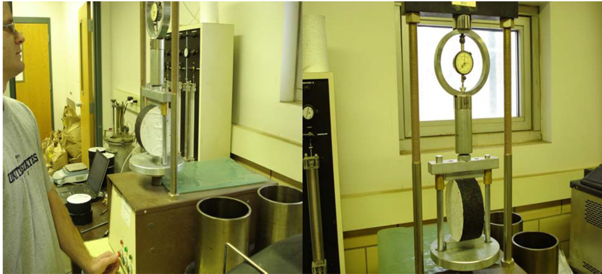
Figure 3-17: Indirect-tensile strength (ITS) testing setup.
