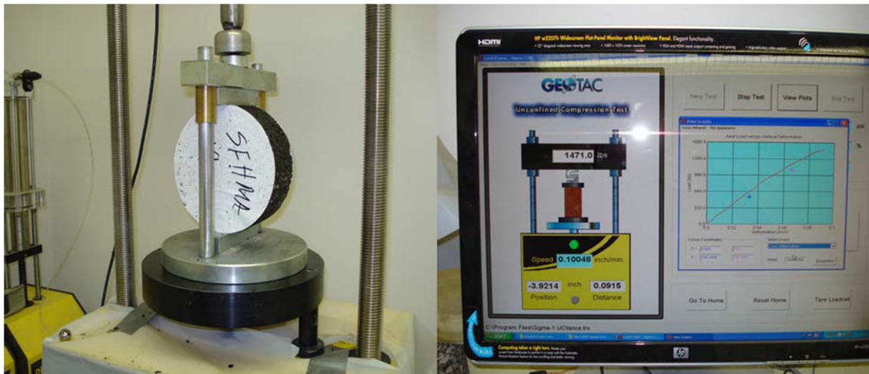
Figure 3-19: C* energy measurement testing setup.
