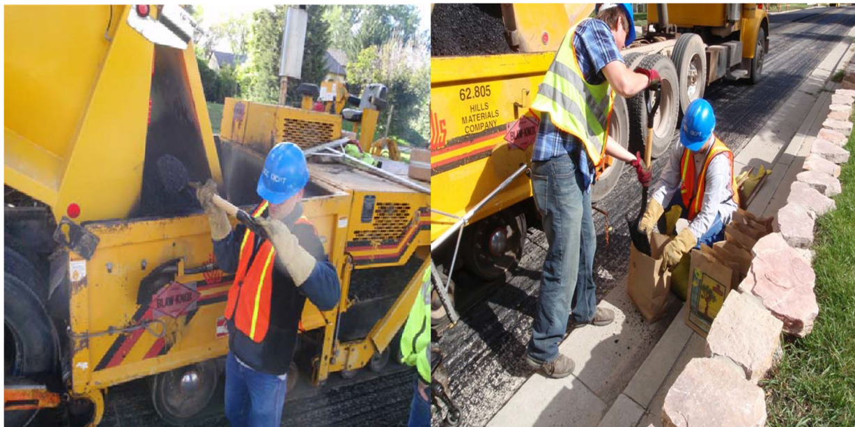
Figure 2-8: Sampling of fiber reinforced HMA material at test section site.
