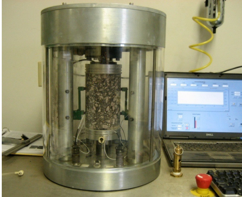
Figure 3-26: Dynamic modulus specimen assembled in SPT machine.
