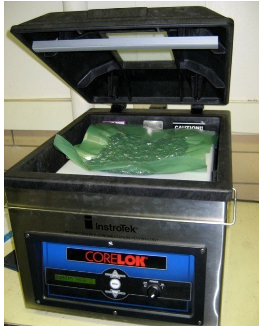
Figure 3-20: Maximum theoretical specific gravity sample in CoreLok device.
