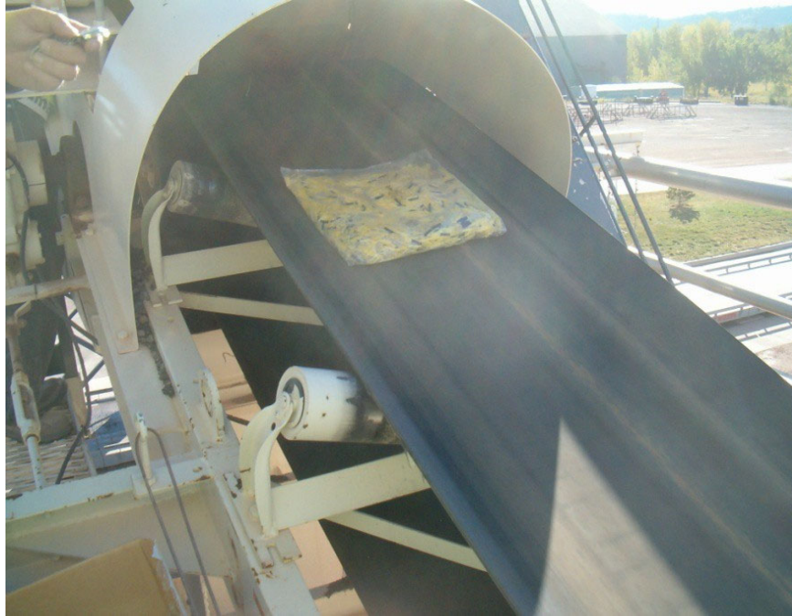
Figure 2-15: Adding the fibers onto the RAP conveyor during asphalt production.
