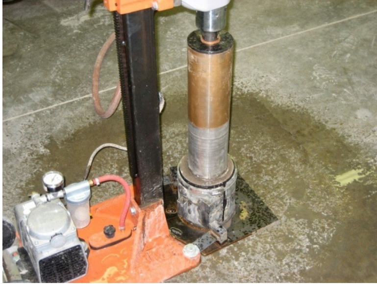
Figure 3-22: HMA coring operation.
