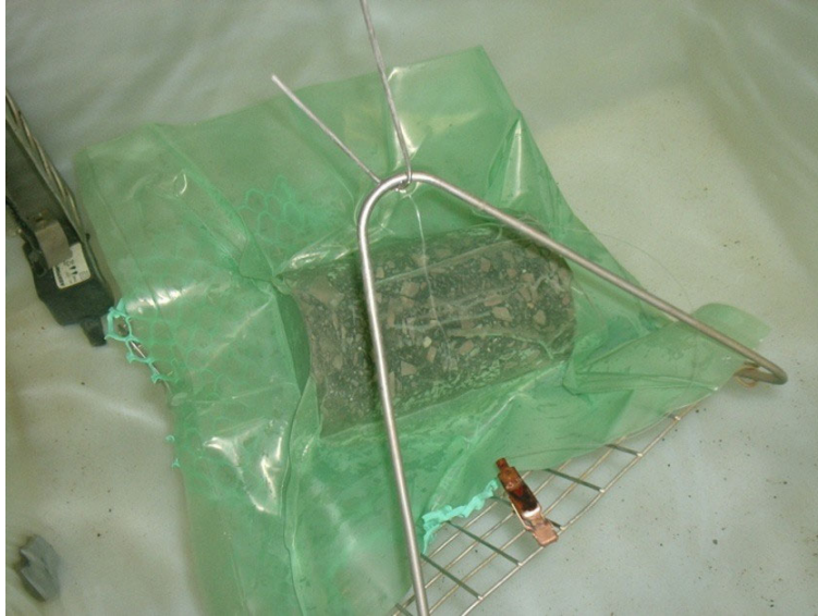
Figure 3-24: Submerged HMA sample for bulk specific gravity determination.
