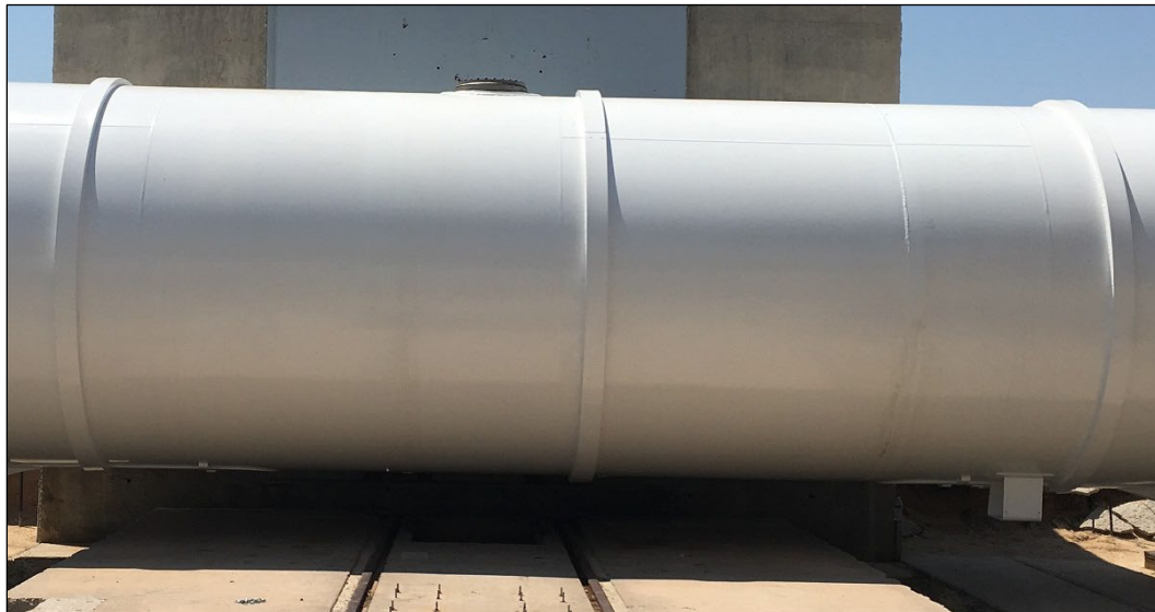
Figure 10. Tank Car Reinforcement Rings
