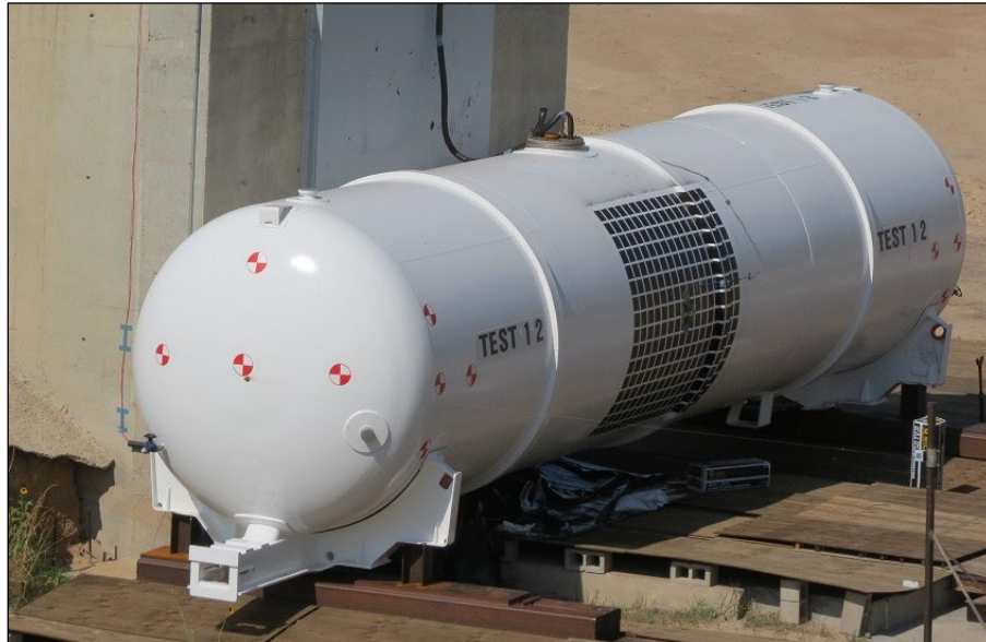
Figure 1. DOT-113 Surrogate Tank Car Mounted on Support Skids
