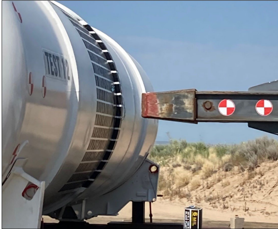
Figure 9. Ram Arm with 12-inch by 12-inch Indenter Aligned with Impact Zone on the Tank Car
