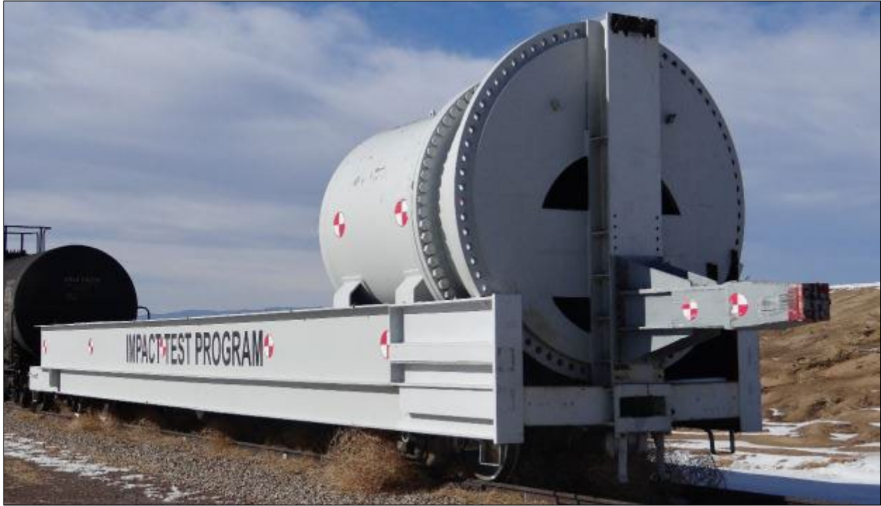
Figure 7. Ram Car and Head
