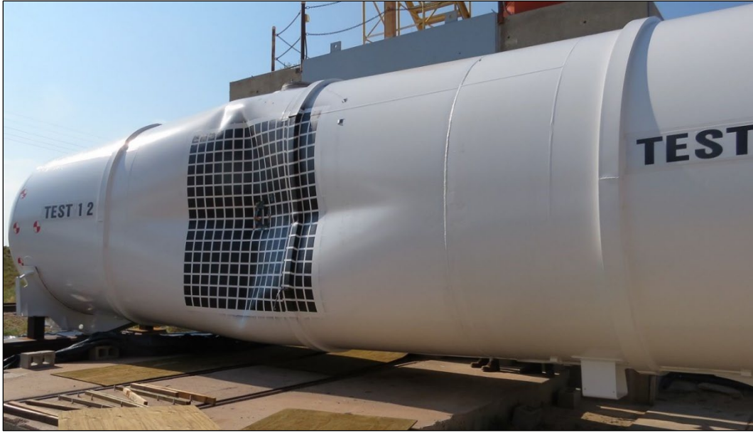
Figure 22. Tank Car after the Impact (impact side)
