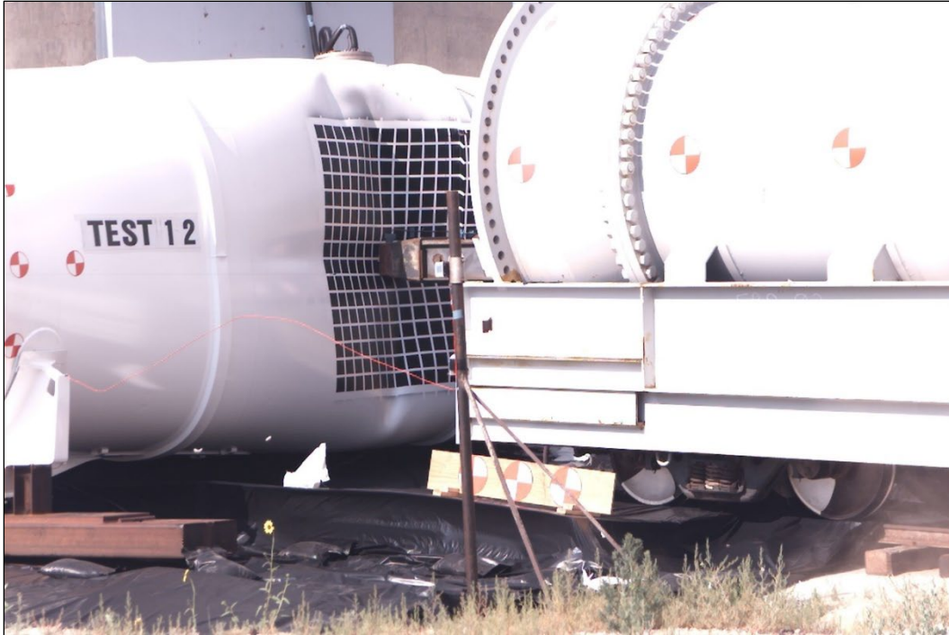
Figure 25. Still Frame from HS Video Taken at Approximate Time of Maximum Indentation (0.308 seconds)
