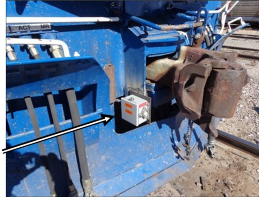
Figure 8 – Locomotive end box on short hood end
