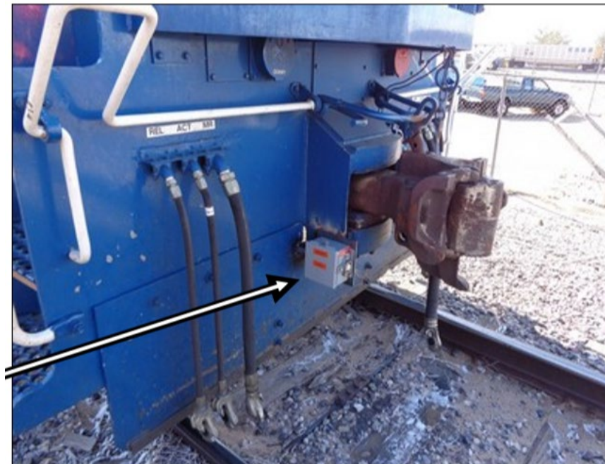
Figure 9 – Locomotive end box on long hood end
