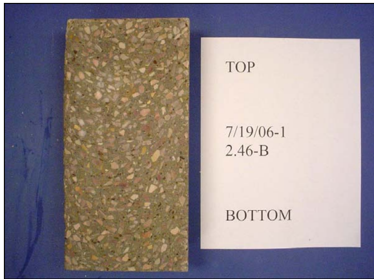
Figure 7.58: Sawn Concrete Cylinder made with Limestone (Western South Dakota) Aggregates
