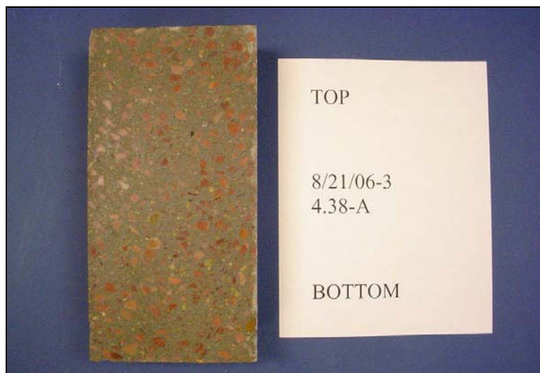
Figure 7.59: Sawn Concrete Cylinder made with Quartzite (Eastern South Dakota) Aggregates
