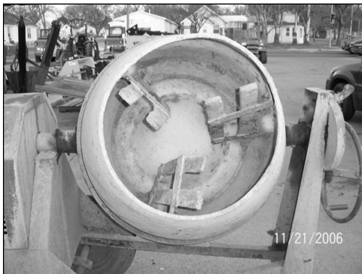
Figure 7.9: The Concrete Mixer Used for Preparing the SCC Laboratory Batches
