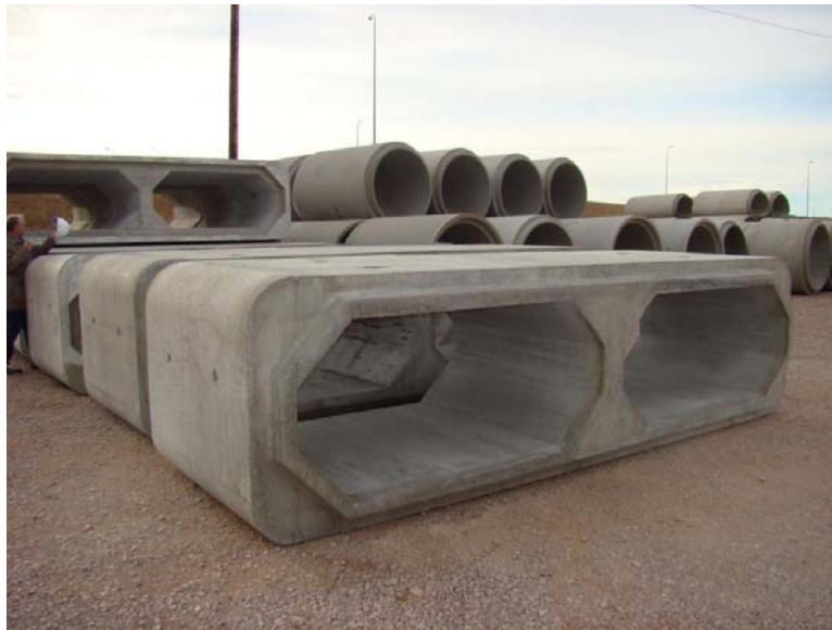
Figure 8.3: Completed SCC Box Culvert Units
