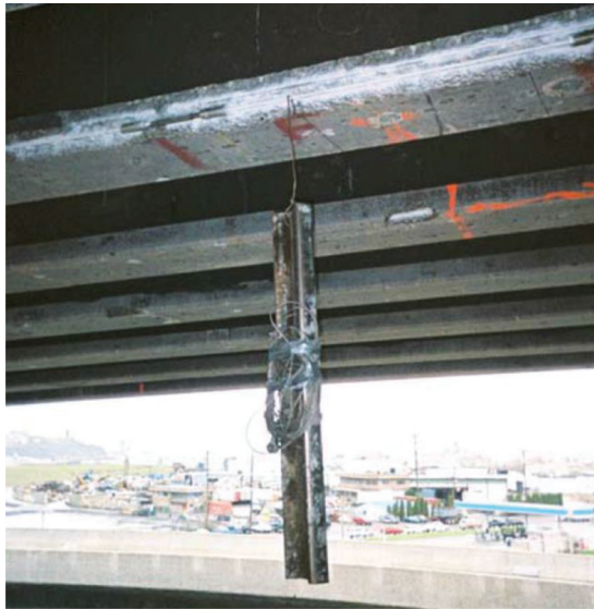
Figure 3.5 Deflection test on exposed strand (Stoddard, 2004).
