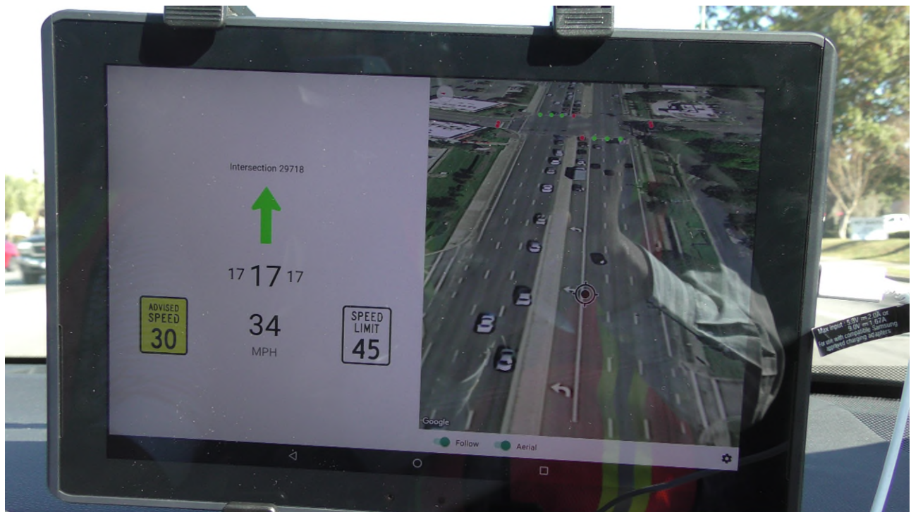
Figure 2.6 Display of SPaT Information on the Screen
