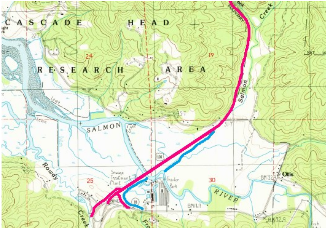
Figure 1.5: Map highlighting the relocated US 101 (wide pink lines) and changes to the course of Salmon Creek and Frazer Creek (wide blue lines)
