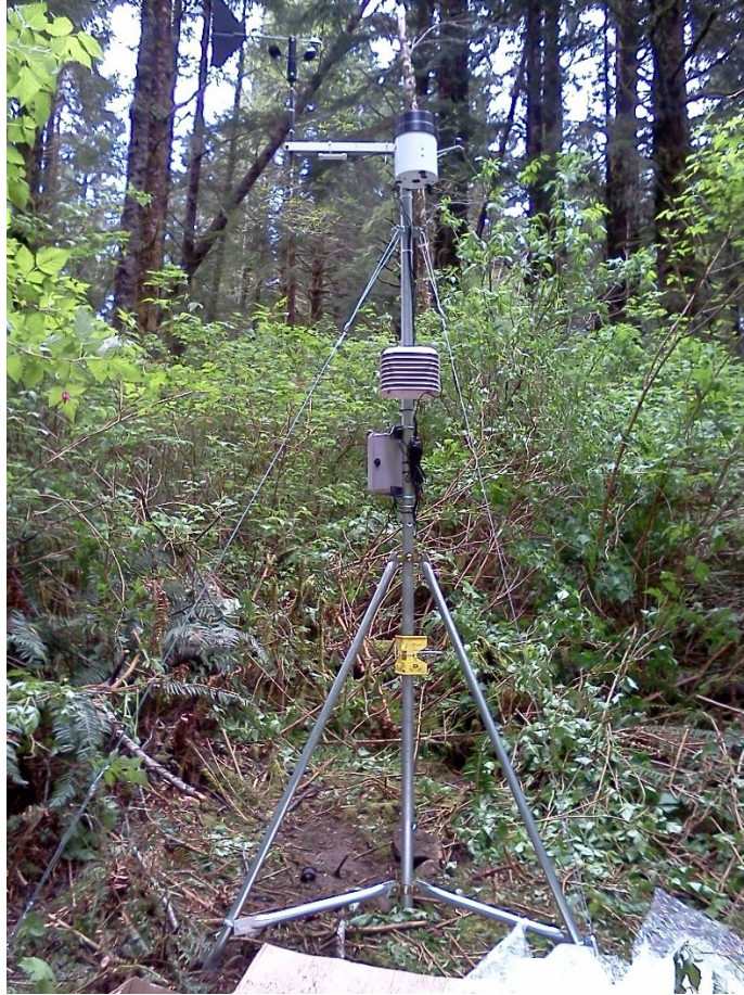
Figure 3.27: Highlands Weather Station equipment.
