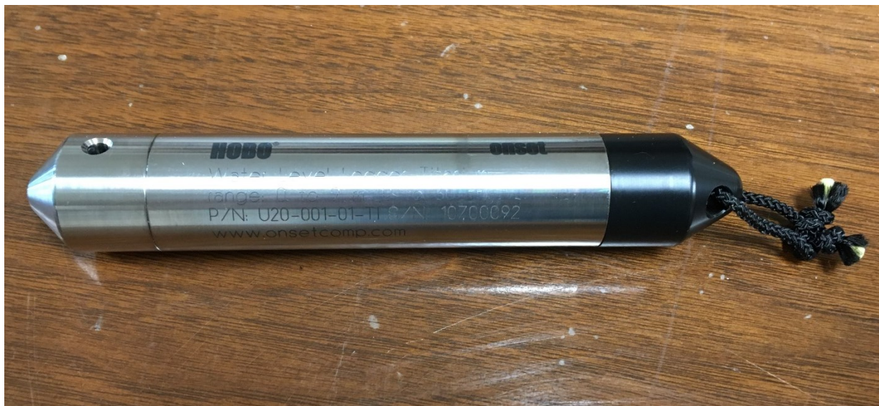
Figure 2.3: Onset HOBO U20Ti Water Level Logger device.
