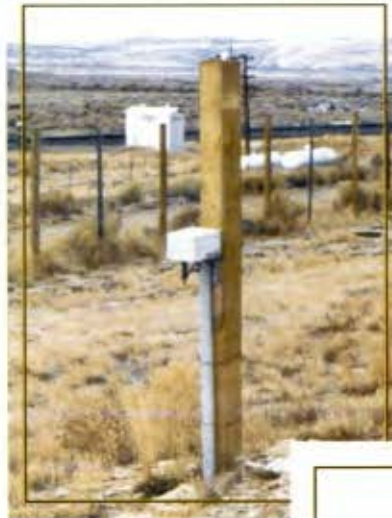
Microwave radar mounted just outside the boundary fence pointed into the crossing zone. Visible in the background is the one-way jump over. One is located on each side of the crossing zone and on both sides of the highway. Most deer walked or trotted straight through the crossing, but occasionally they would drift or be driven by traffic to one side or another on the highway. These sites channeled the deer off the highway where they would use the jump area where the dirt was sloped toward the fence in the corner.
