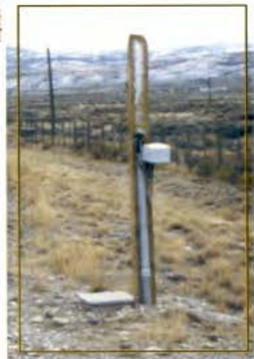
Microwave radar mounted just outside the boundary fence pointed into the crossing zone. Visible in the background is the one-way jump over. One is located on each side of the crossing zone and on both sides of the highway. Most deer walked or trotted straight through the crossing, but occasionally they would drift or be driven by traffic to one side or another on the highway. These sites channeled the deer off the highway where they would use the jump area where the dirt was sloped toward the fence in the corner.
