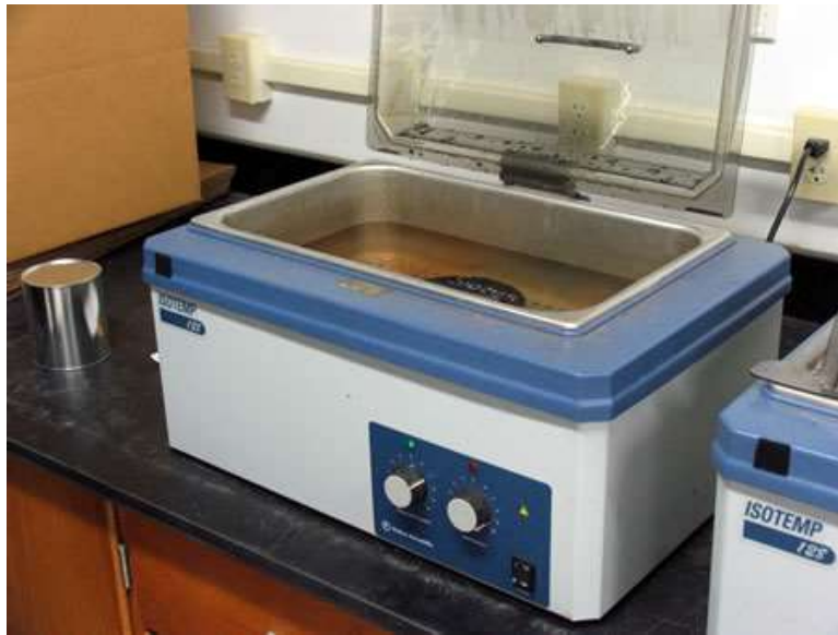
Figure 22: Lottman Temperature Controlled Water Bath (Image from pavementinteractive.org)
