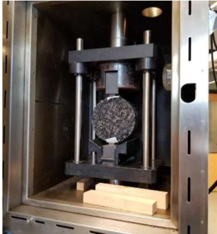
Figure 11: Indirect Tensile Strength Test Fixture
