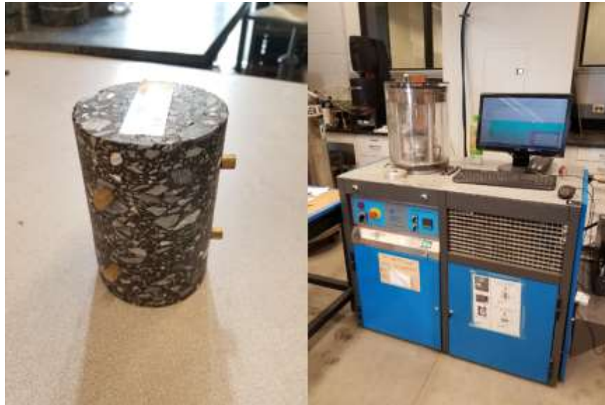
Figure 12: Dynamic Modulus Specimen (Left), AMPT Device (Right)
