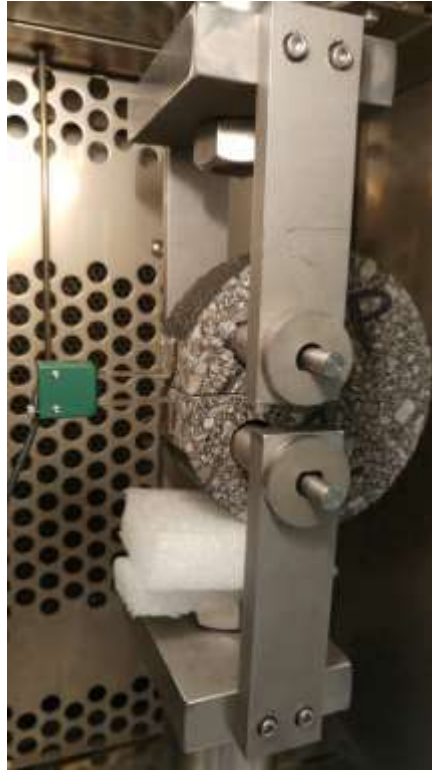
Figure 17: DCT Test Setup on Hydraulic Load Frame
