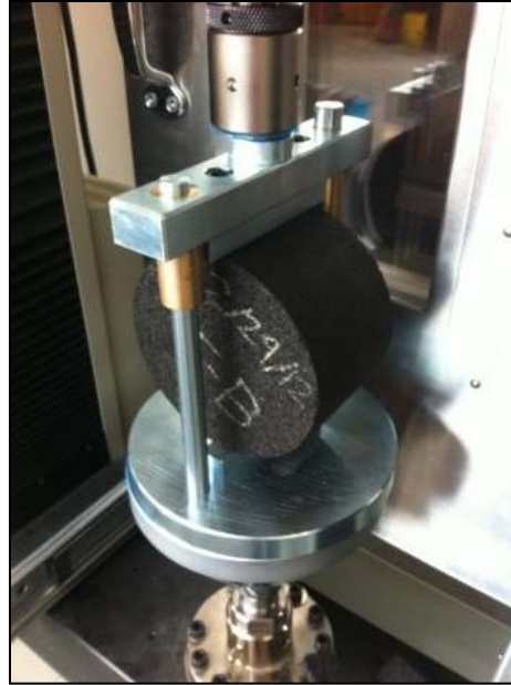
Figure 4: Indirect Tensile Strength Setup
