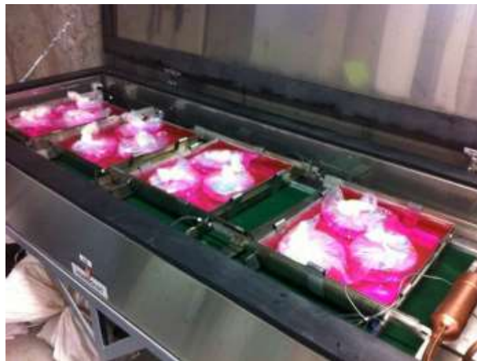
Figure 2: Multi-Cycle Freeze-Thaw Conditioning Set Up
