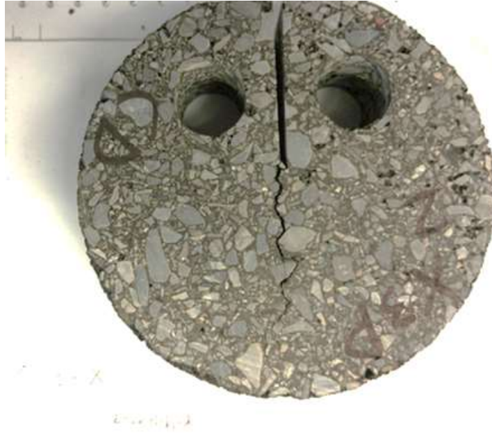
Figure 15: DCT Test Specimen
