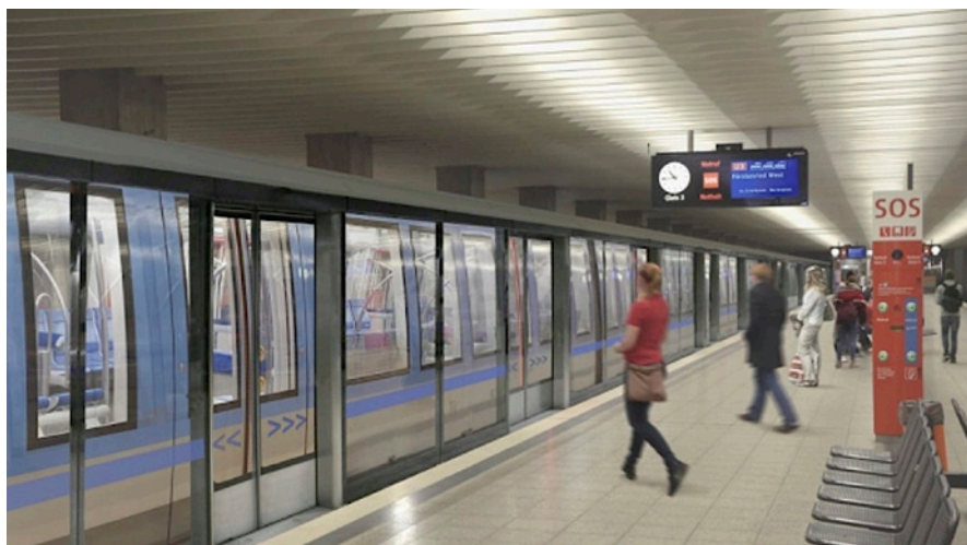
Figure 2-9 Rail infrastructure modification – platform screen doors
