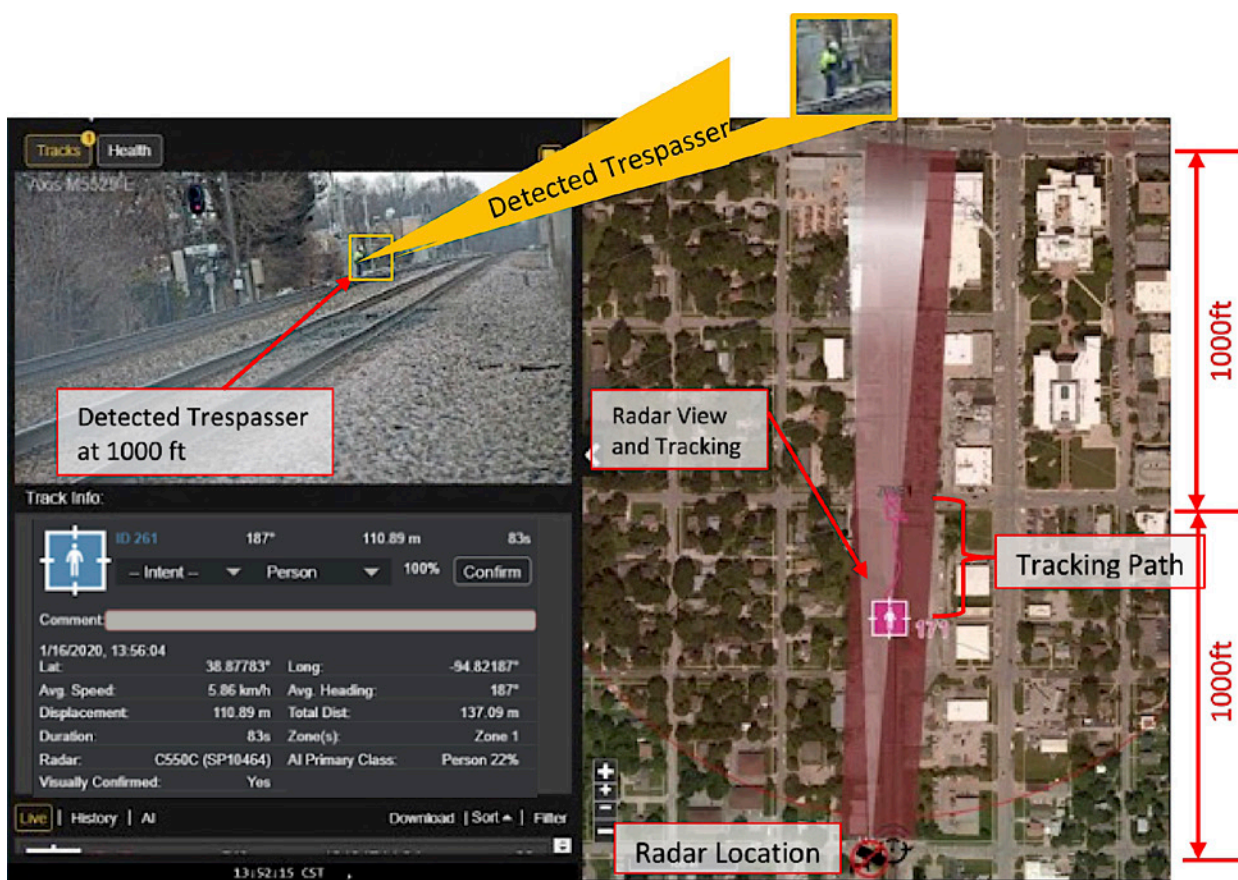
Figure 3-12 Trespasser detection – long-range radar
