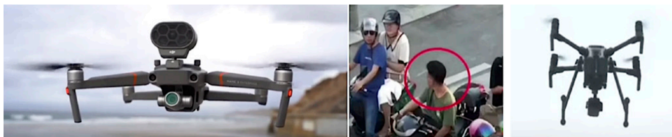
Figure 3-11 Examples of aerial drone applications with loudspeaker to warn surfer and motorcyclist
