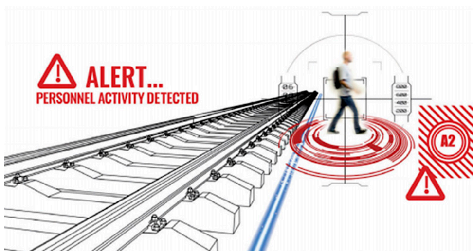
Figure 3-5 Trespasser detection – fiber-based sensor device
