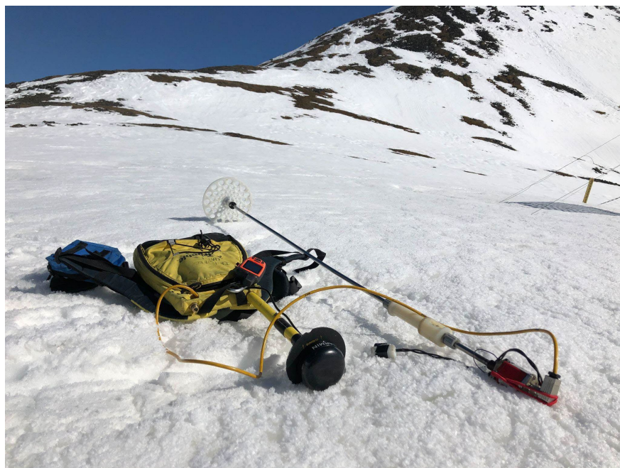
Figure 4.7 Magnaprobe equipment in Atigun Pass on May 20, 2020
