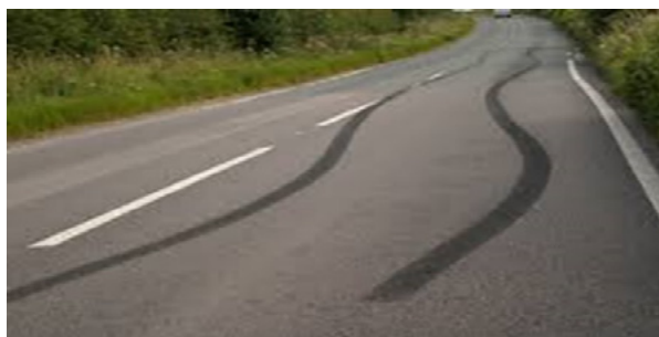
Figure B-17 Acceleration Marks
