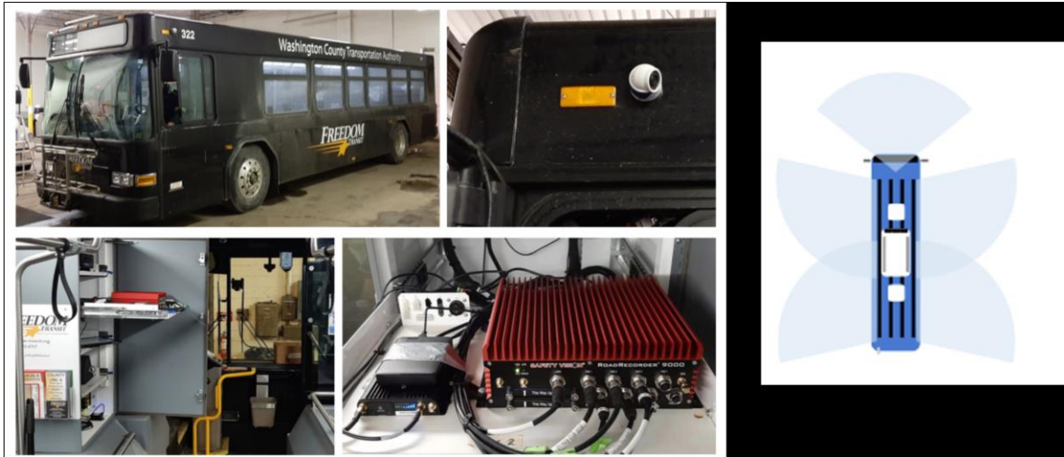
Figure 1 The left four images show the commuter bus, an image of the camera, the cabinet that contains the computer and electronics, and one of the cameras. The right diagram shows the field of view of each installed camera, where one faces forward and four side cameras face opposite directions from each other.
