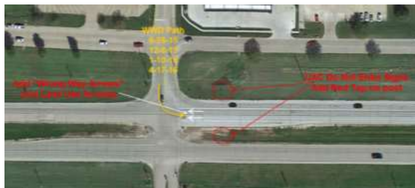
Improvements at Linn Street and U.S. 30 Intersection: DNE Signs on Both Sides of Highway, Wrong-Way Arrow Pavement Markings (Source: Iowa DOT)
