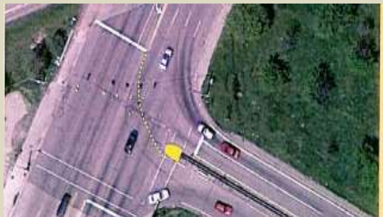
Skip Lines to Guide Drivers onto Entrance Ramp, Stop Bar at End of Exit Ramp (Source: Morena & Leix, 2012)
