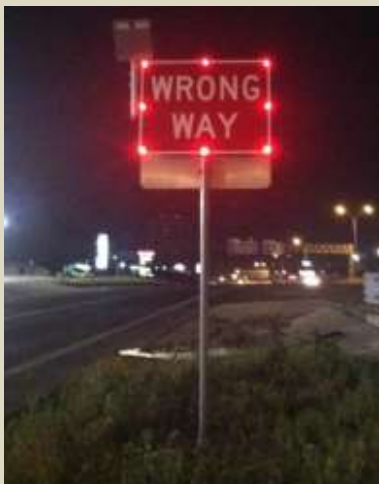
LEDs at WRONG WAY Sign Border, Flash Continuously at Night & Low Light (Source: Provided by Texas DOT)
