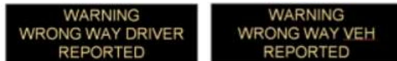
DMS Messages to Oncoming Right-Way Traffic Left Image: Recommended; Right Image: Alternative 15-character Message (Source: Finley, et al., 2016)
