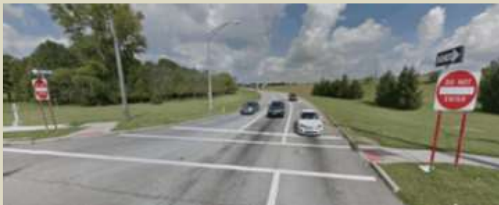
One Way Signs Mounted over DNE Signs (Source: Provided by Ohio DOT)
