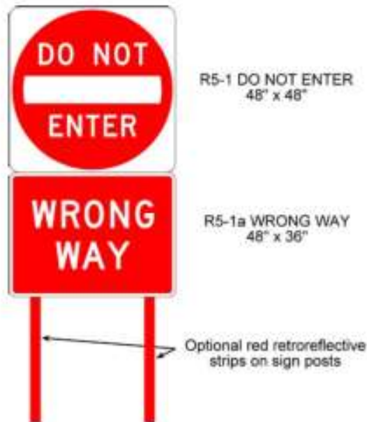
Figure 314-A. DO NOT ENTER / WRONG WAY Sign Assembly
