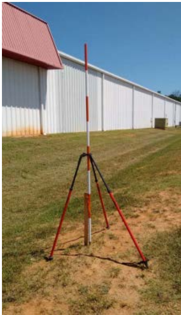
Figure 5-2 Range Pole Set Up at an SCP
