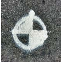
Figure 6-2 Painted target with PK nail in center
