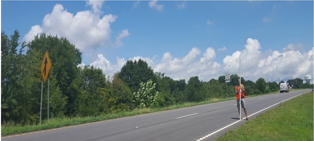
Figure 3-2 Field Surveying at the Six Stations (Sign Locations)
