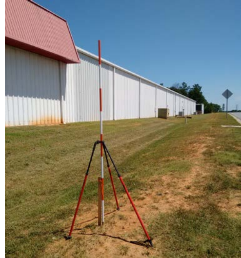
Figure 4-4 Range Pole Location
