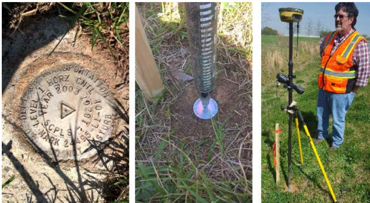
Figure 4-1 Primary and Secondary GCPs and Using Dual Frequency Topcon GPS on Section 2
