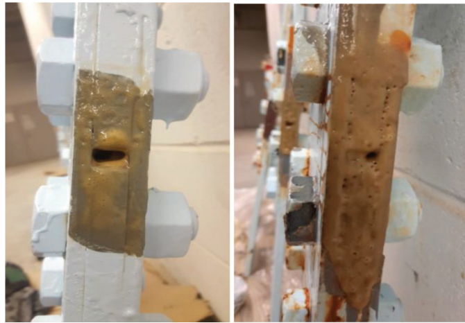
Figure 4.20 Fluid Film application for initial and repair condition.
