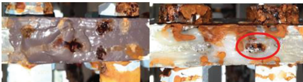
Figure 5.1 Black rust in Termarust (left) and caulked (right) specimens for Condition A.
