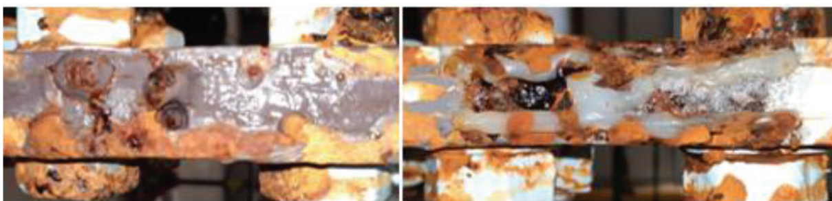
Figure 5.3 Black rust in Termarust (left) and caulked (right) specimens for Condition B.
