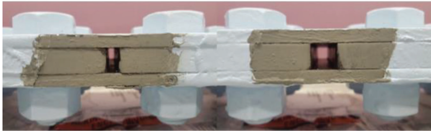
Figure 4.15 Close up image of the 1/4-inch gap specimen and 1/2-inch gap specimen.
