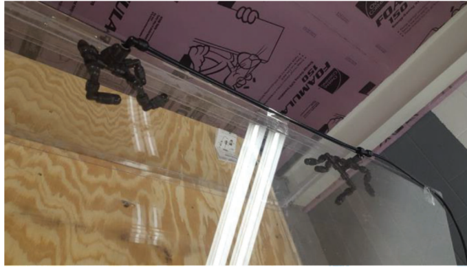
Figure 4.4 Roof of Lexan boxes holding the atomizers.
