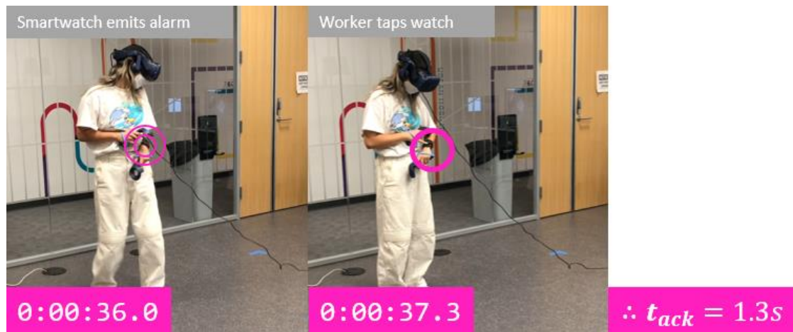
Figure 9: Illustration of how watch response/acknowledgement time is calculated
