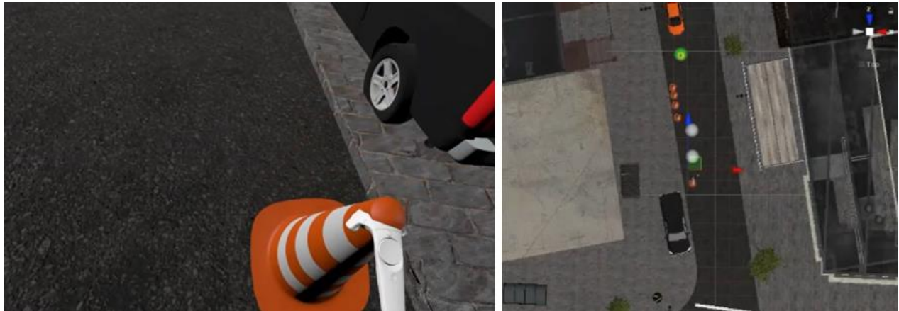
Figure 2: Screenshot of Unity3D worker’s VR perspective (left) and bird’s eye view (right). Note the red and blue arrows on the right top corner, which indicate the X-axis and Z-axis location of the worker in the VR environment
