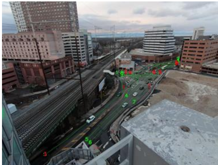
Figure 22. The scanline-based image recognition algorithm
