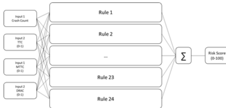
Figure 24. Structure of the fuzzy logic model
