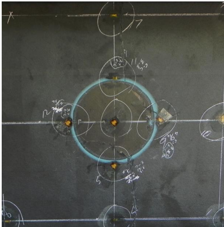
Figure E-8. Panel 10 patch and net section failure, internal surface
