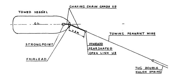
FIGURE 1 EXAMPLE OF TANKER TOWED FROM THE BOW
