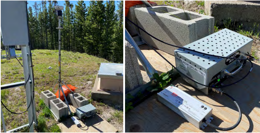
Figure 12: RTK Base Station in the Canyon Village Area
