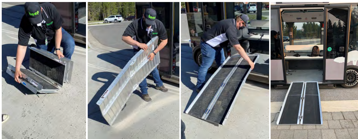
Figure 6: Deployment of Automated Shuttle Accessibility Ramp
