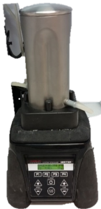
Figure F-7 Set blender agitation speed to 10,000 rpm, and start cycle for 30 seconds.
