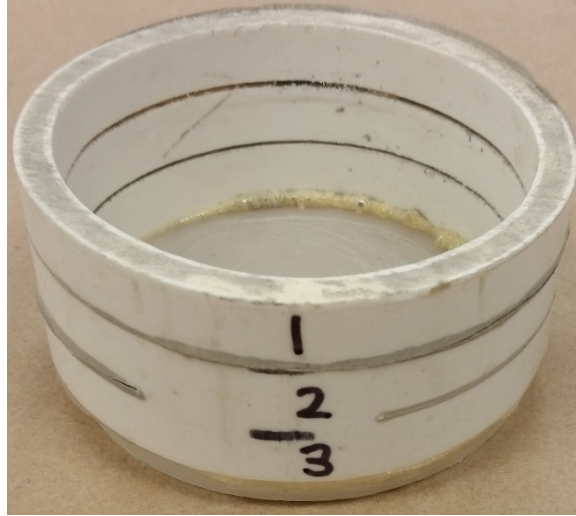
Figure B-2 Small-scale container used for LOI depth-layered testing
