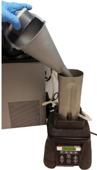
Figure F-6 Pour cementitious material over a 60-second period.
