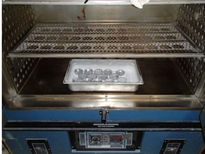
Figure J-17 Moisture content samples inside oven
