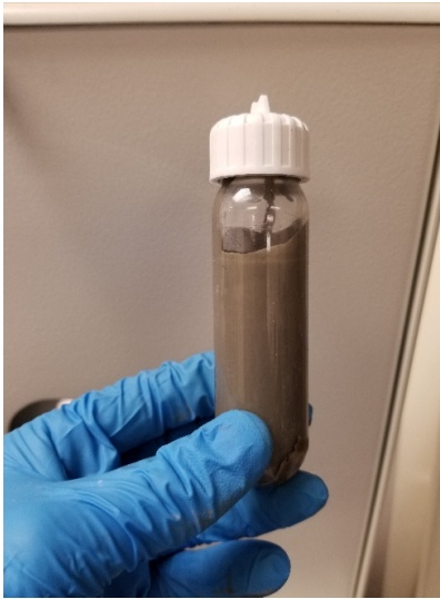
Figure 8-4 Centrifuge tube containing 30 mL of cement paste
