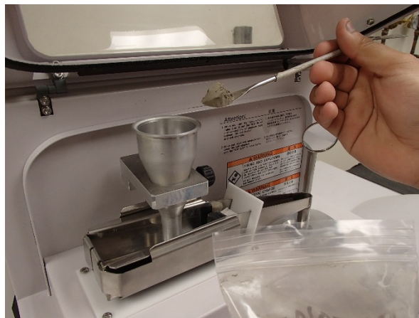
Figure H-4 Place 5 to 10 grams of grout into the hopper.
