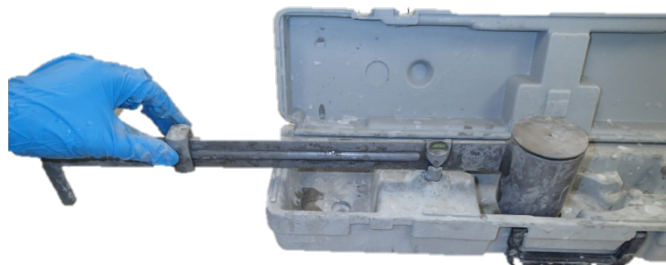
Figure J-6 ASTM C185 “Mud-balance” test
