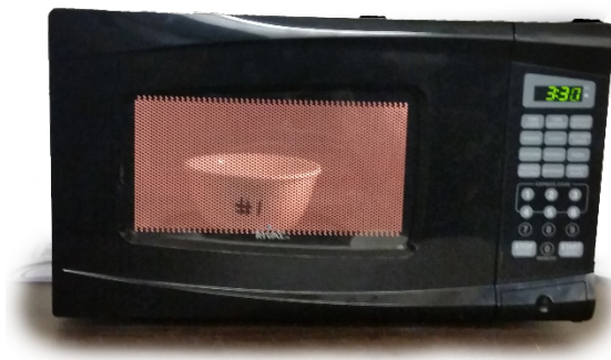
Figure E-1 Microwave used for Moisture Content of cementitious material
