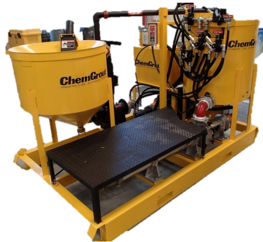
Figure I-1 Chemgrout CG600 E/H – 3CL6 Progressive cavity pump
