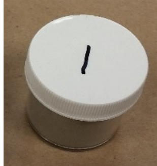
Figure 6-2 Plastic containers used for LOI layered-material sampling
