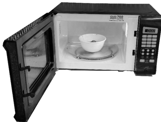
Figure 15-1 Microwave Moisture Content Test
