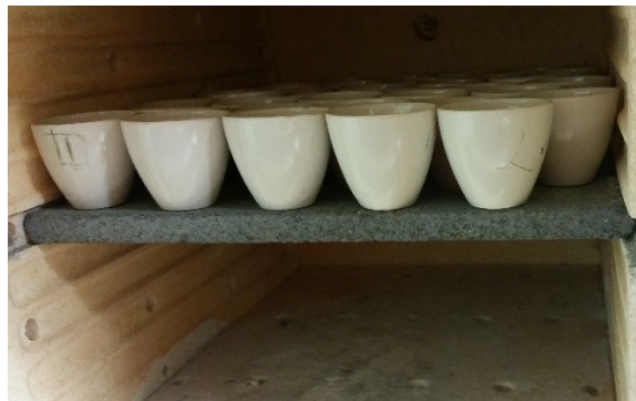
Figure D-5 Add crucible to furnace at 550°C.
