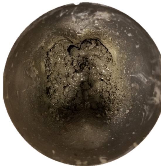
Figure 8-14 A3 mixture after mixing shows lack of fluidity after 10 days of exposure.
