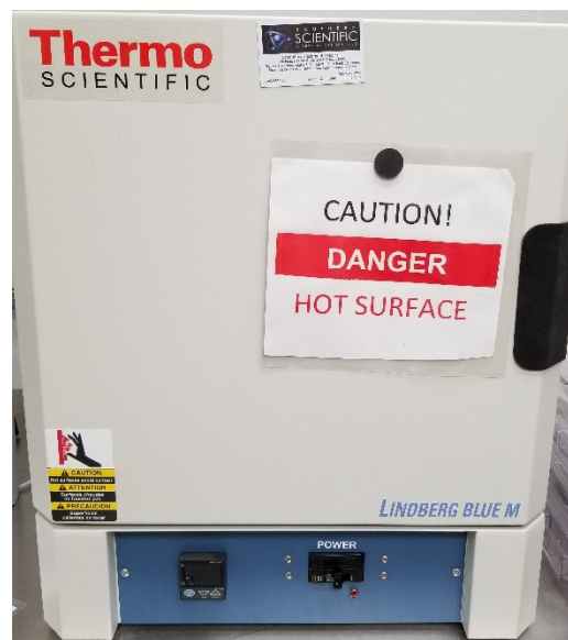
Figure 13-1 Loss on Ignition testing furnace
