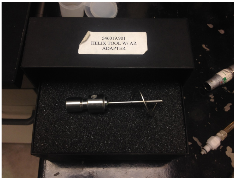
Figure G-5 Stainless steel helical rotor
