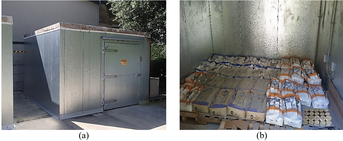
Figure 5-3 Walk-in chamber used to impose the Field exposure on grout and cement
