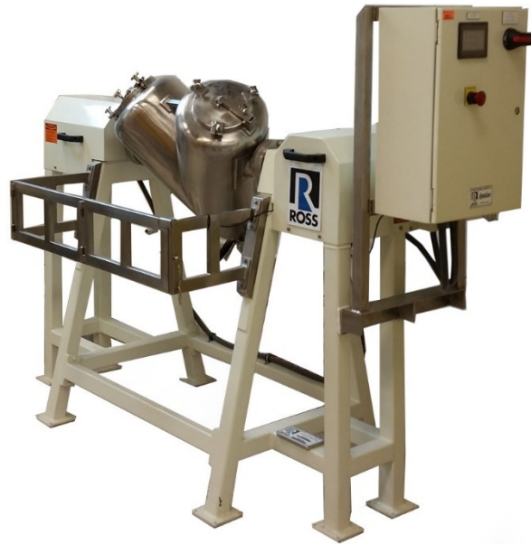
Figure A-1 Ross V-Blender Model VCB-1 SN#110960 – 2-HP driving motor and 1-HP Intensifier motor
