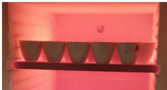
Figure D-6 Remove crucible from the furnace after 3 h at 950°C.
