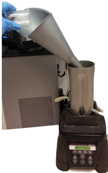
Figure F-5 Pour water into blender, and start cycle.
