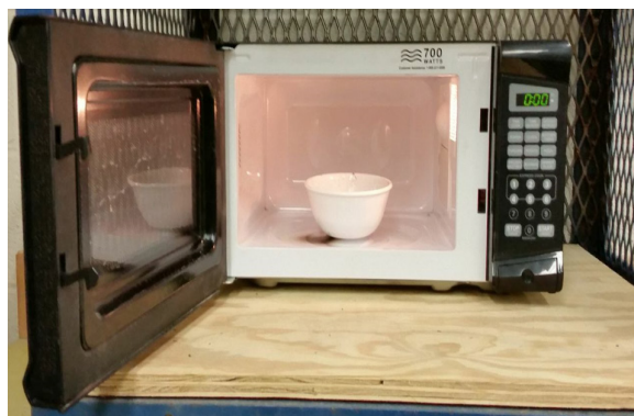
Figure E-5 Place container with sample in the microwave, and begin heating cycle.
