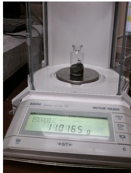
Figure 9-5 Weight of PT grout for isothermal calorimetry
