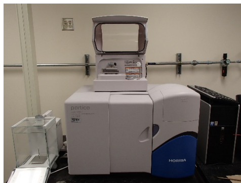
Figure H-1 HORIBA LA-950V2 Laser-Scattering Particle Size Distribution Analyzer
