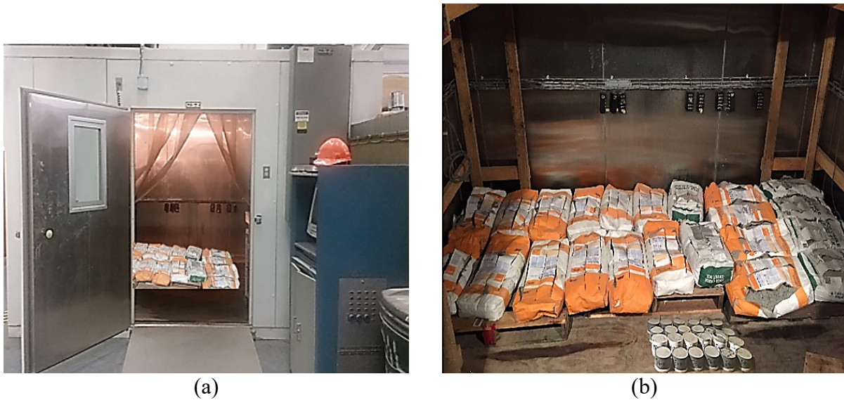
Figure 5-4 Walk-in chamber used to impose the Extreme exposure on grout and cement
