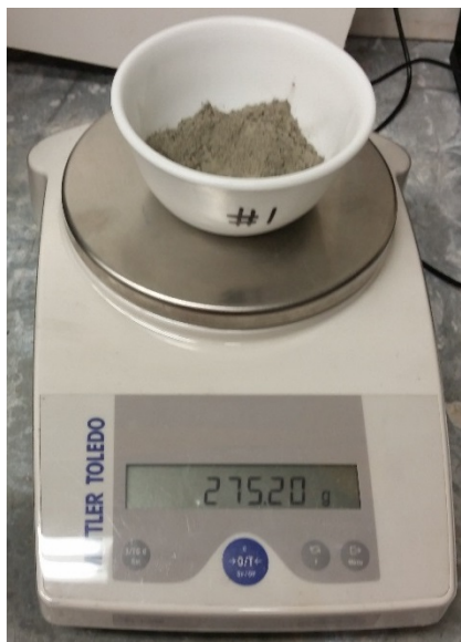
Figure E-4 Measure initial cementitious material mass.
