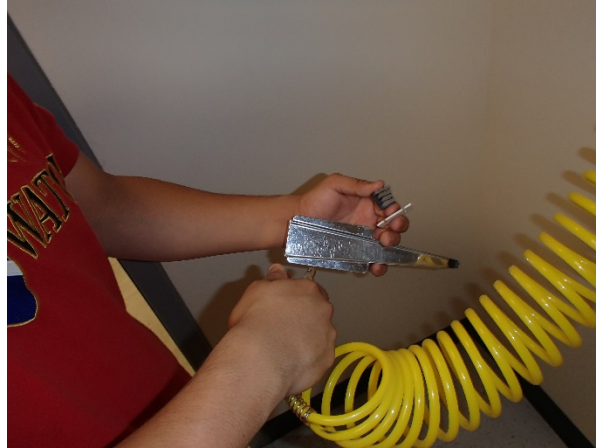
Figure H-5 Cleaning the hopper with compressed air
