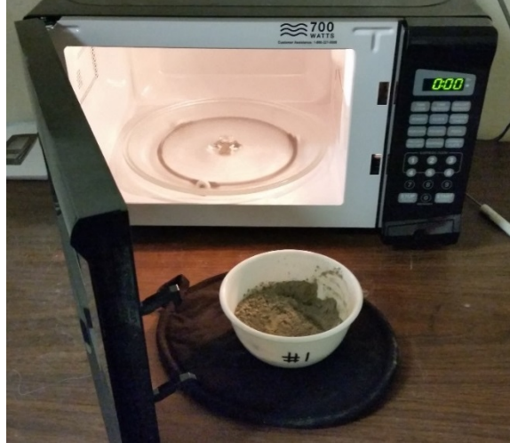
Figure E-6 Remove specimen from microwave with heat-resistant apparatus.
