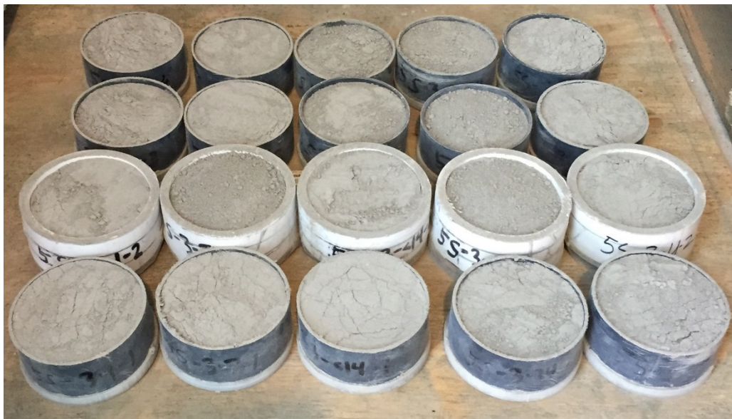
Figure B-1 Small-scale containers used to in mass gain testing
