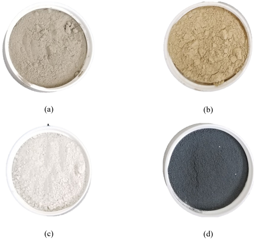
Figure 4-1 SCMs tested: (a) Fly ash class F (FAF), (b) Fly ash class C, (c) Slag (S), and (d) Silica fume (SF)
