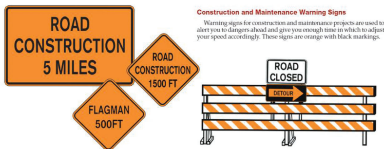
Figure 2.6 Construction and maintenance warning signs, Georgia’s MO.
