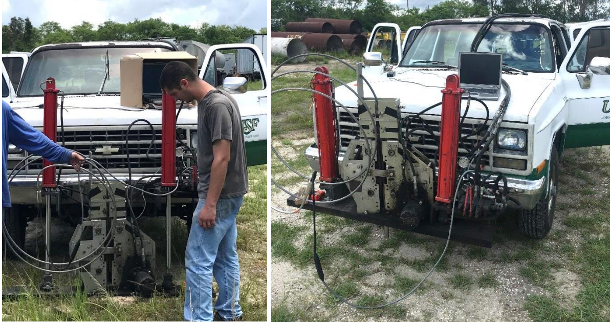
Figure 4.3 Cone penetration testing at Clearwater test site.
