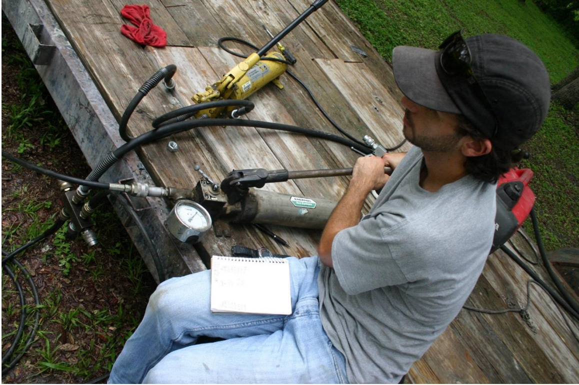
Figure 3.55 Operation of hand pump during static load test.
