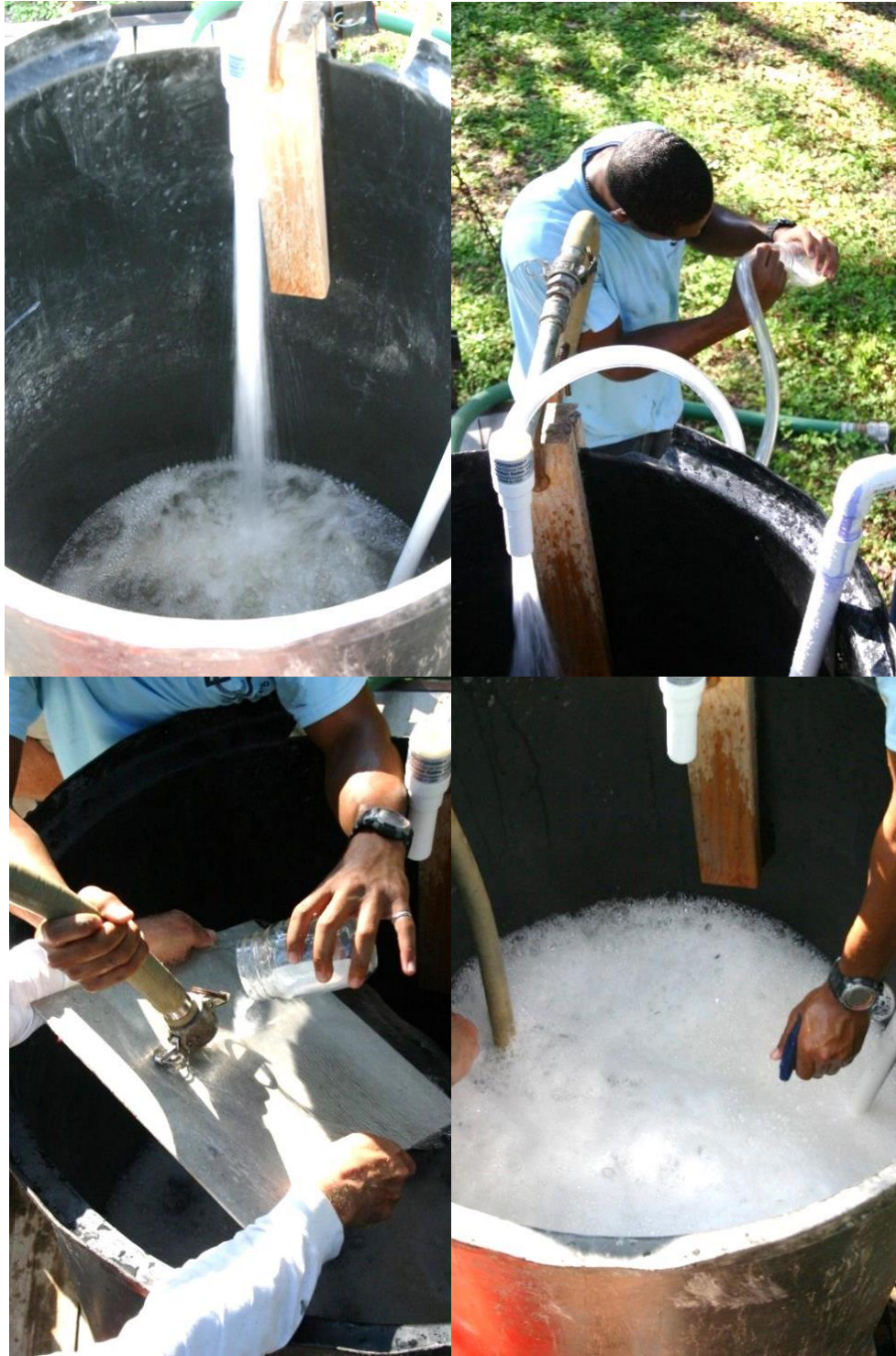
Figure 3.29 Hootonanny™ eductor (top left), vacuuming dry product with eductor (top right), Enhanceit100 introduction with spill plate (bottom left), spraying of MPA after all dry products were added (bottom right).
