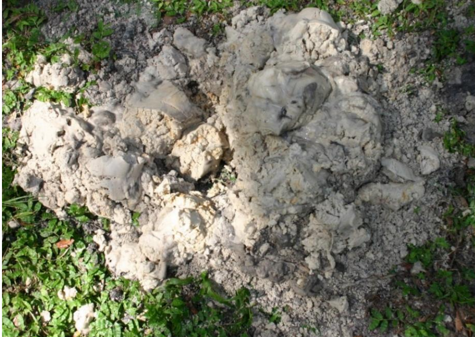
Figure 3.86 Soils excavated with Cetco ShorePac polymer.
