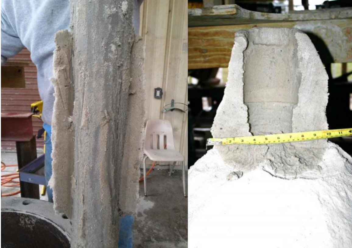
Figure 1.1 Bentonite filter cake and wetted soil around model shaft (left), polymer stabilized soil around same size model excavation (right).
