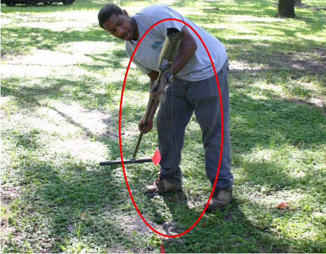
Figure 3.74 Matrix Bigfoot polymer chains hanging from auger during emptying.
