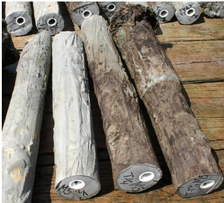
Figure 3.82 Exposed concrete surface (left) next to soil laden surface (right) for matrix polymer shafts.
