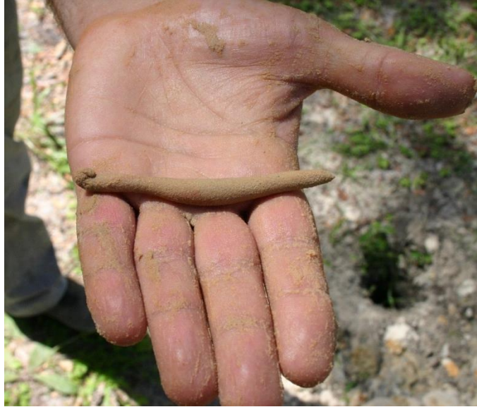
Figure 3.78 Excavated material rolled to confirm clay-like properties.
