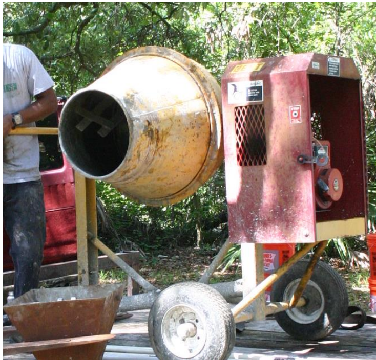
Figure 3.9 Gas-powered concrete mixer discharging to tremie hopper.
