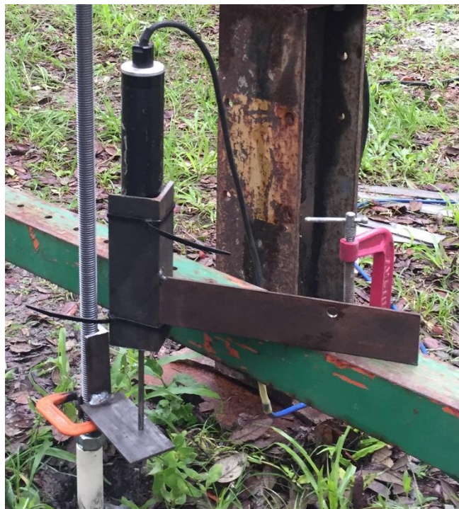
Figure 3.25 Mounted LVDT, bracket and displacement tab.
