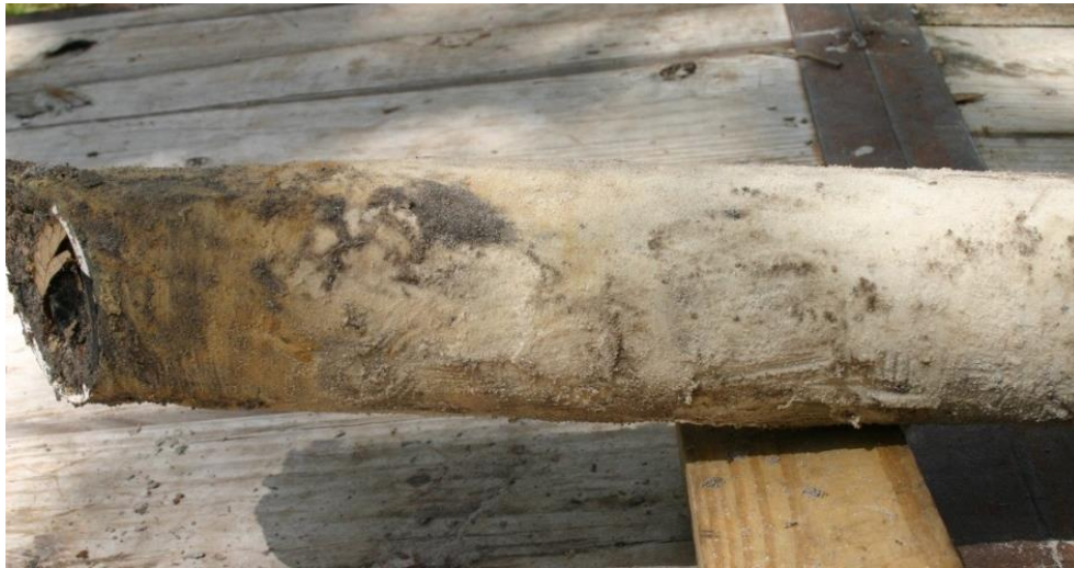
Figure 3.65 Bottom 2ft of extracted KB International Enhanced CDP shaft.
