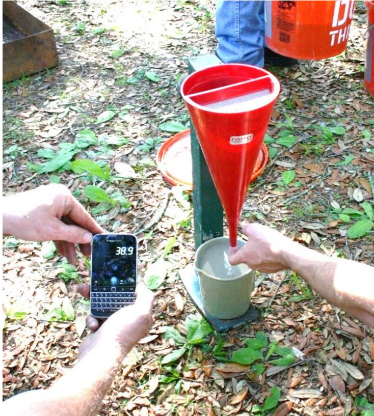
Figure 3.44. Marsh funnel viscosity field test.
