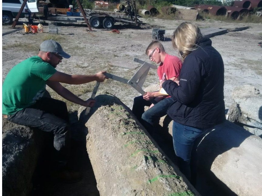
Figure 4.31 Caliper used to take diameter measurements of each shaft.
