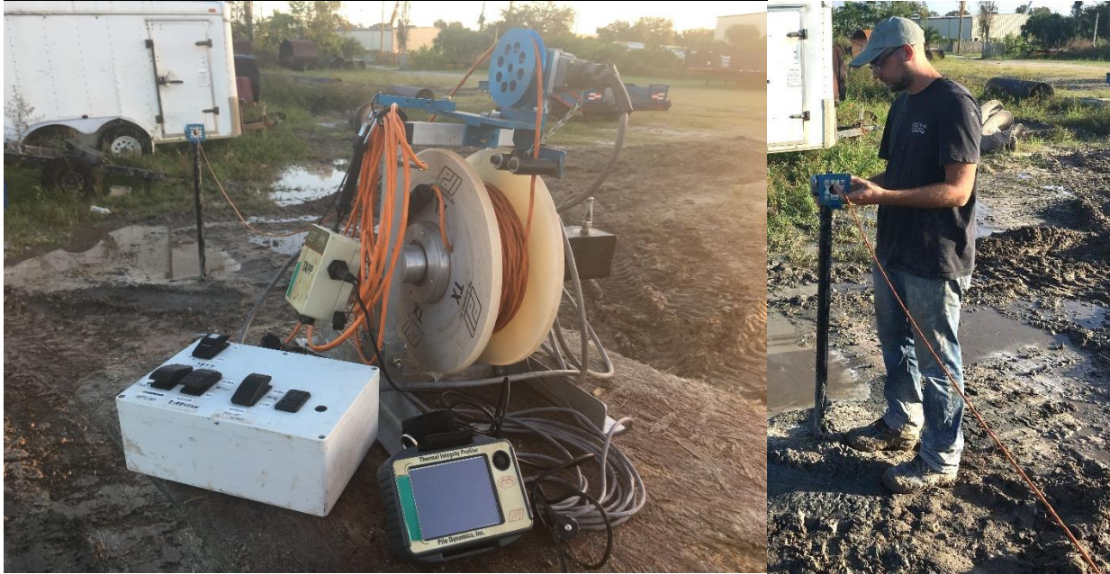
Figure 4.24 Thermal probe testing using automated reel system starting immediately after casting.
