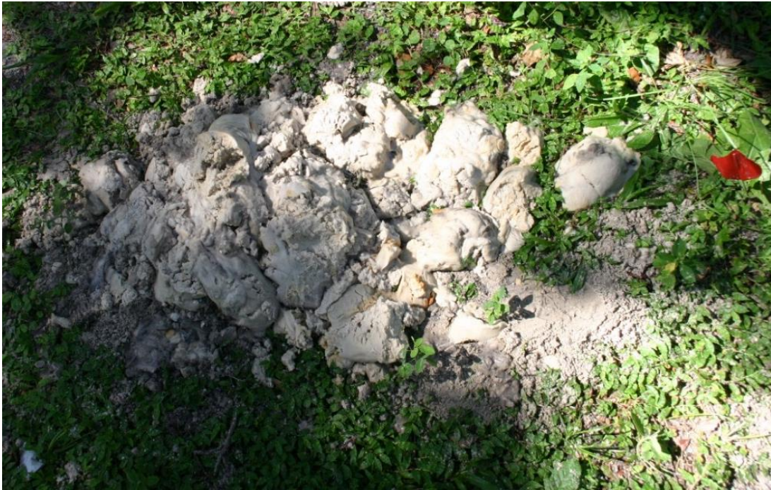
Figure 3.75 Soil excavated with Matrix Bigfoot polymer.
