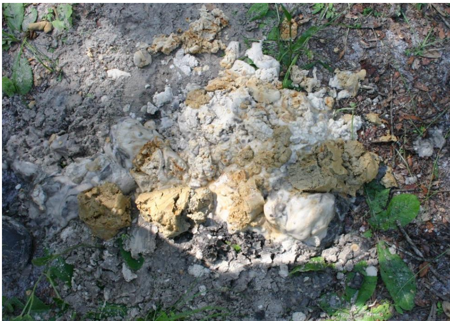
Figure 3.77 Clayey soils encountered at bottom of Matrix polymer shafts.
