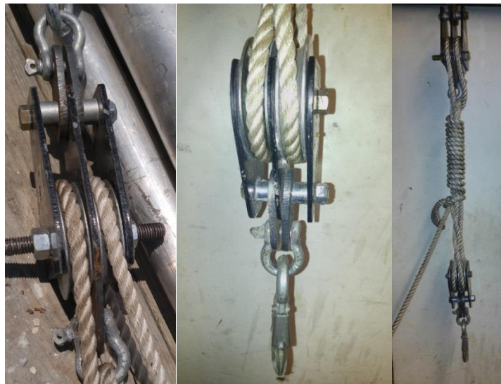
Figure 3.19 Standing block (left), travelling block (middle), stored block and tackle (right).
