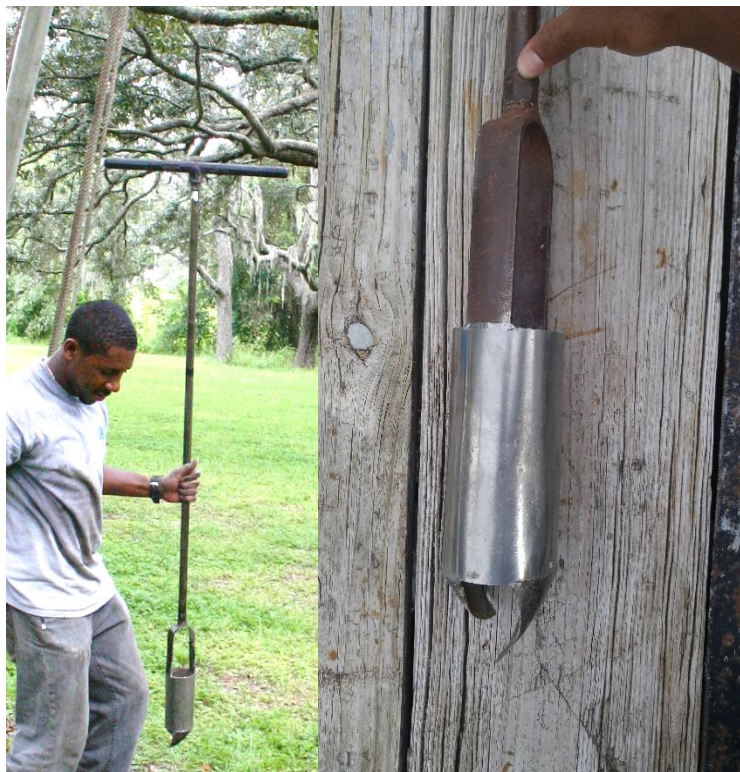
Figure 3.5 hand auger (left) and close-up of drilling bucket (right).
