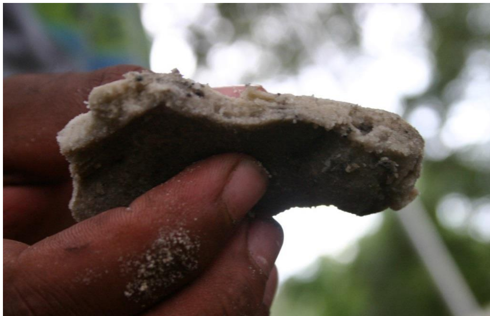
Figure 3.66 "Soil Cake" of saturated soil removed from extracted KB International Enhanced CDP shaft.
