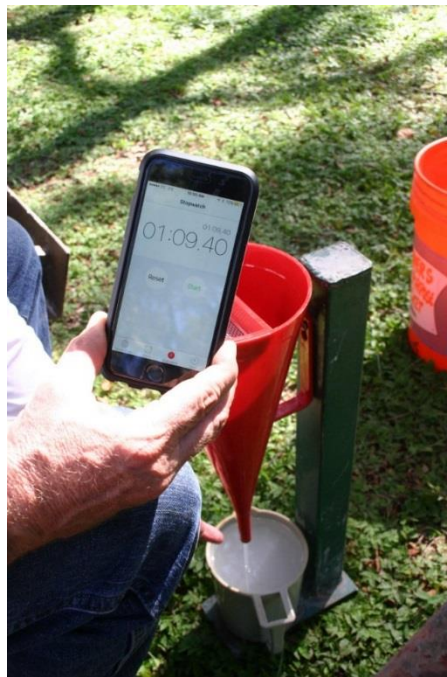
Figure 3.85 Marsh funnel viscosity (70 s/qt).
