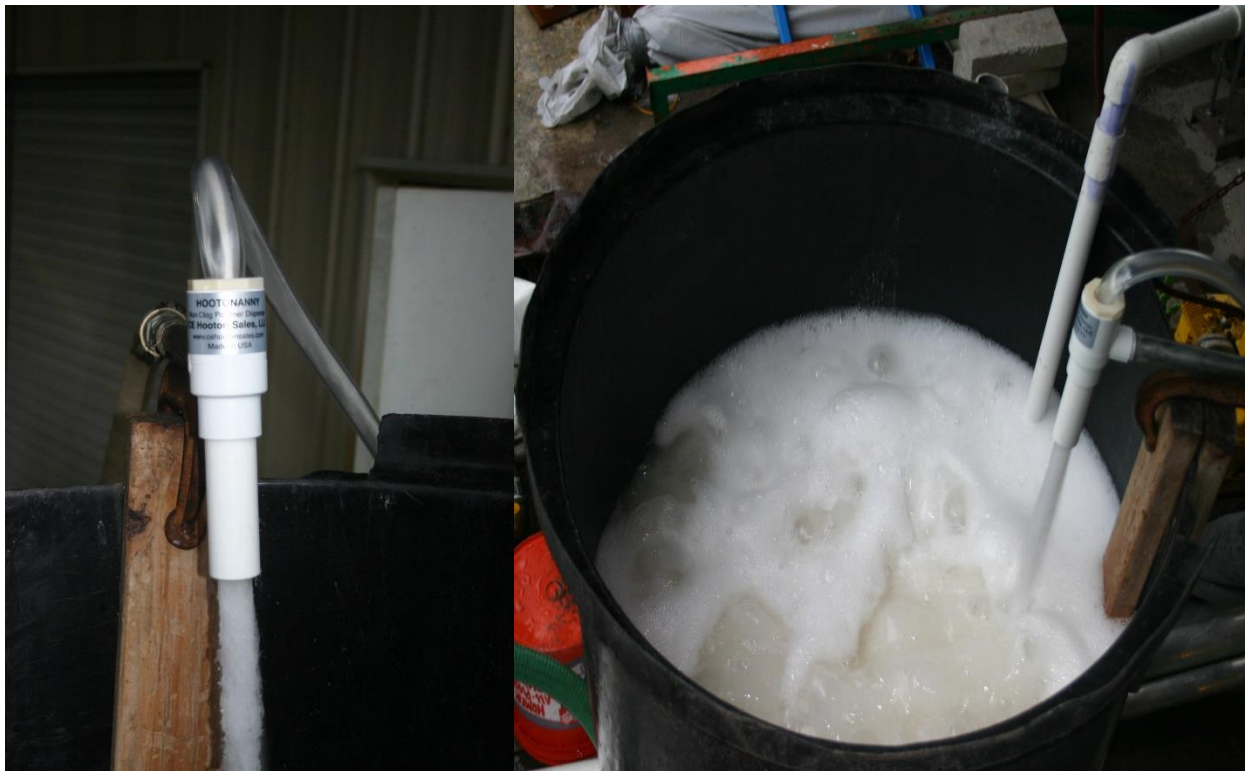
Figure 3.31 Big-Foot product introduction through Hootonanny™ (left), aeration during mixing of Big-Foot polymer system (right).
