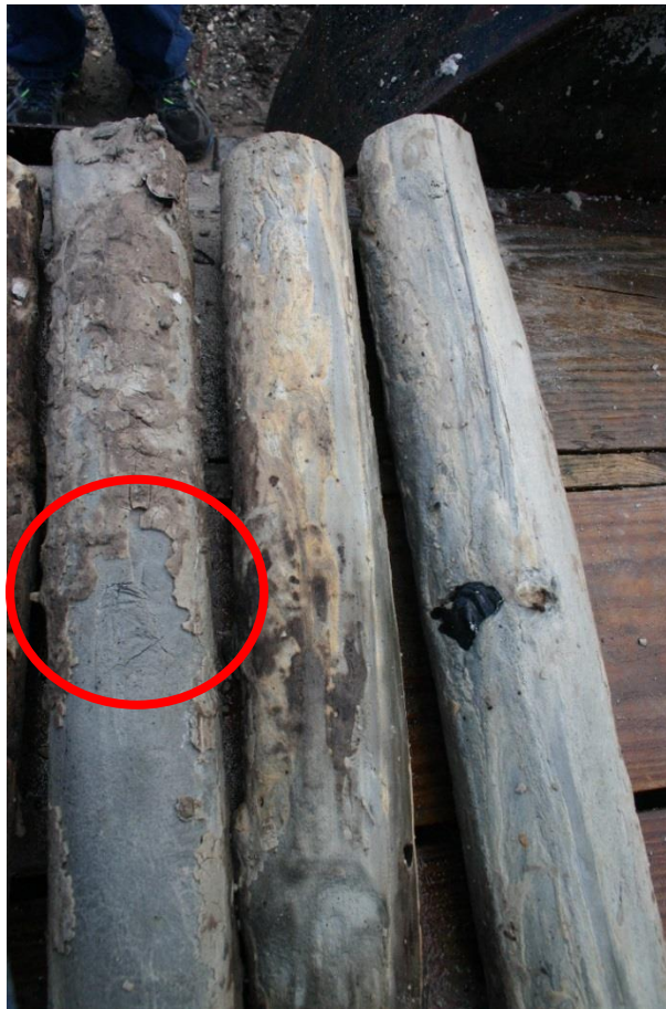
Figure 3.59 Hardened filter cake on bentonite shaft quarters.
