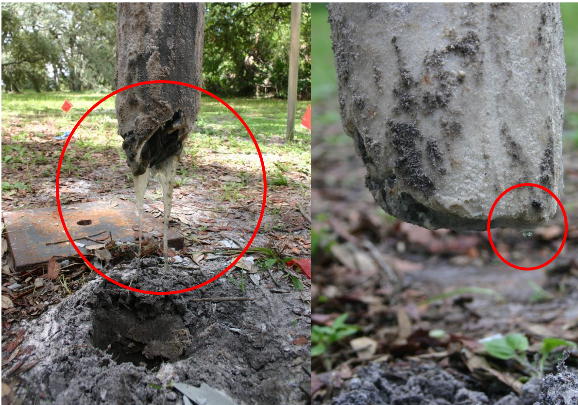
Figure 3.69. Slurry hanging from KB2-8hr shaft (left), drop of liquid on KB3-24hr shaft (right).
