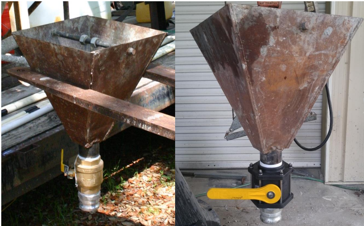
Figure 3.13 Concrete hopper, brass valve (left) and plastic valve (right).
