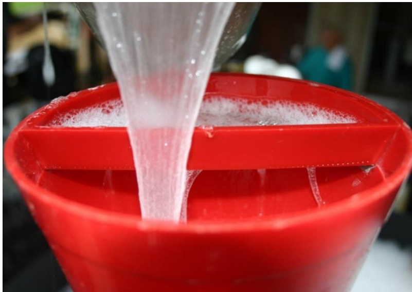
Figure 3.32 Addition of Big-Foot slurry system to Marsh funnel (136sec/qt).
