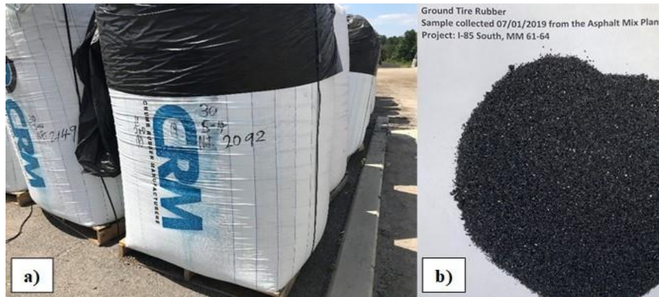
Figure 4. GTR Material: a) on-site storage at plant; b) ground rubber particles. GTR = ground tire rubber.
