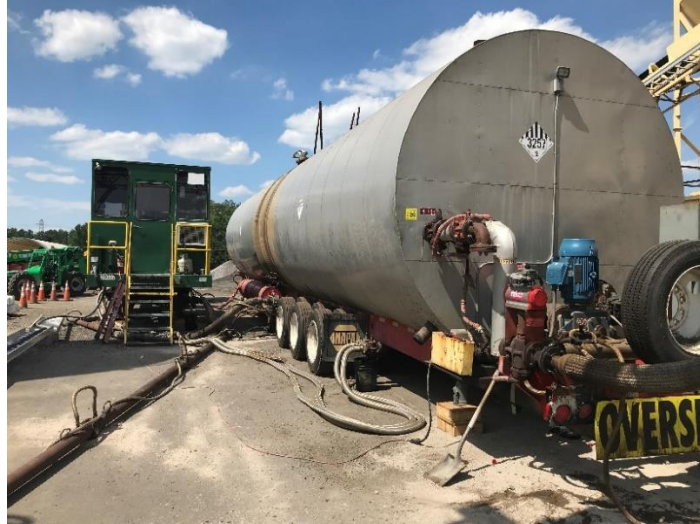
Figure 7. Asphalt Rubber Binder Holding Tank
