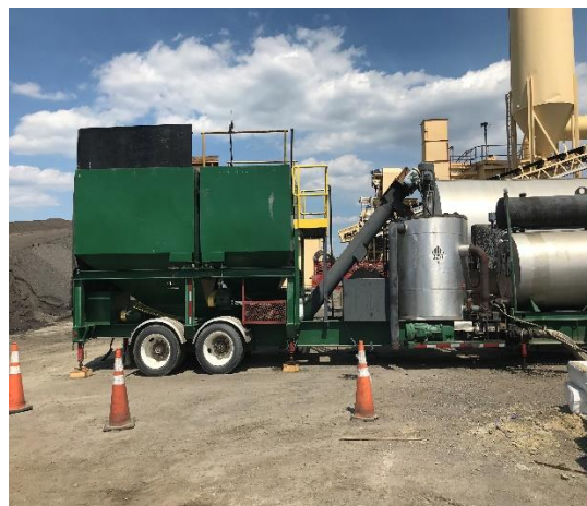
Figure 5. GTR Feed Bins to the Left (Green Bins) and Mixing Tank to the Right (Silver Vertical Tank). GTR = ground tire rubber.
