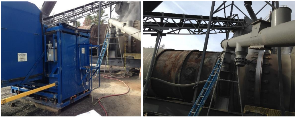
Figure 4. Adding GTR in the Asphalt Plant (Dry Process): left, GTR feeding machine; right, GTR added through the RAP collar. GTR = ground tire rubber; RAP = reclaimed asphalt pavement.
