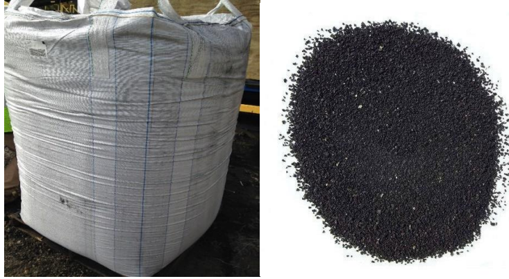
Figure 3. GTR Material: left, GTR stored in bags; right, GTR material in powder form. GTR = ground tire rubber.
