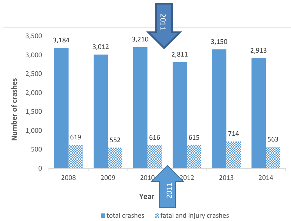
Figure 1.2: Crash Distribution Before and After Speed Limit Change for Freeways Affected by Speed Limit Change
