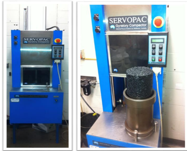
Figure 12. Servopac Gyrotory Compactor and Gyrotory Stability Sample after Compaction
