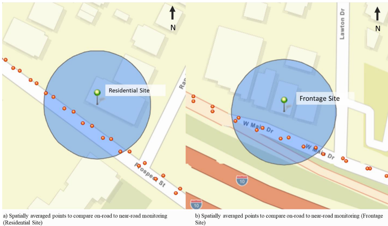
Figure 24 Spatial data points used for estimating hourly average on-road concentration near a stationary site, a) Sunbowl and b) CAMS 12
