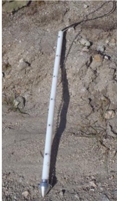
Figure 3. TSDC Probe with Scour Chain
