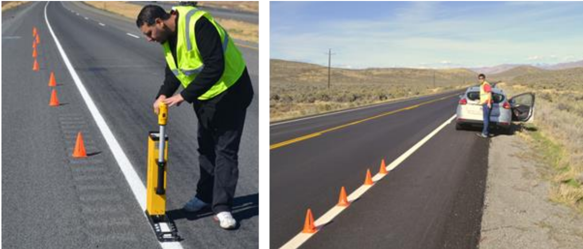
Figure 7 Measuring Retroreflectivity in the Field Test Sites Using the MX 30 Retroreflectometer.
