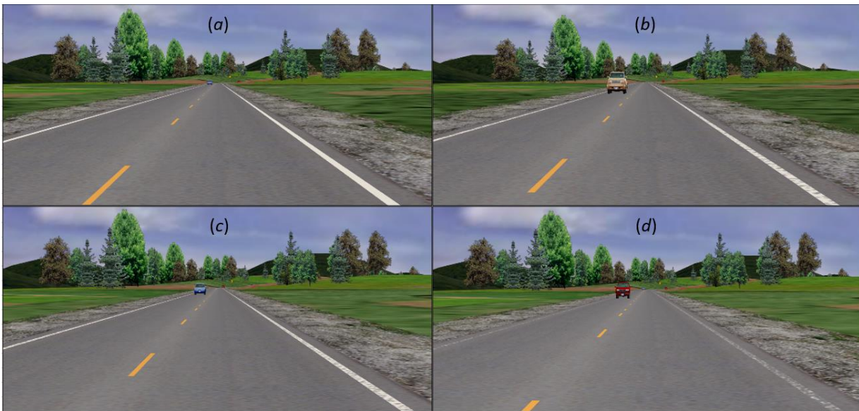
Figure 3 Driver Simulator Graphic of Edge Line Deterioration Percentages (only 6 inch shown): (a) 0 percent, (b) 25 percent, (c) 50 percent, and (d) 75 percent.
