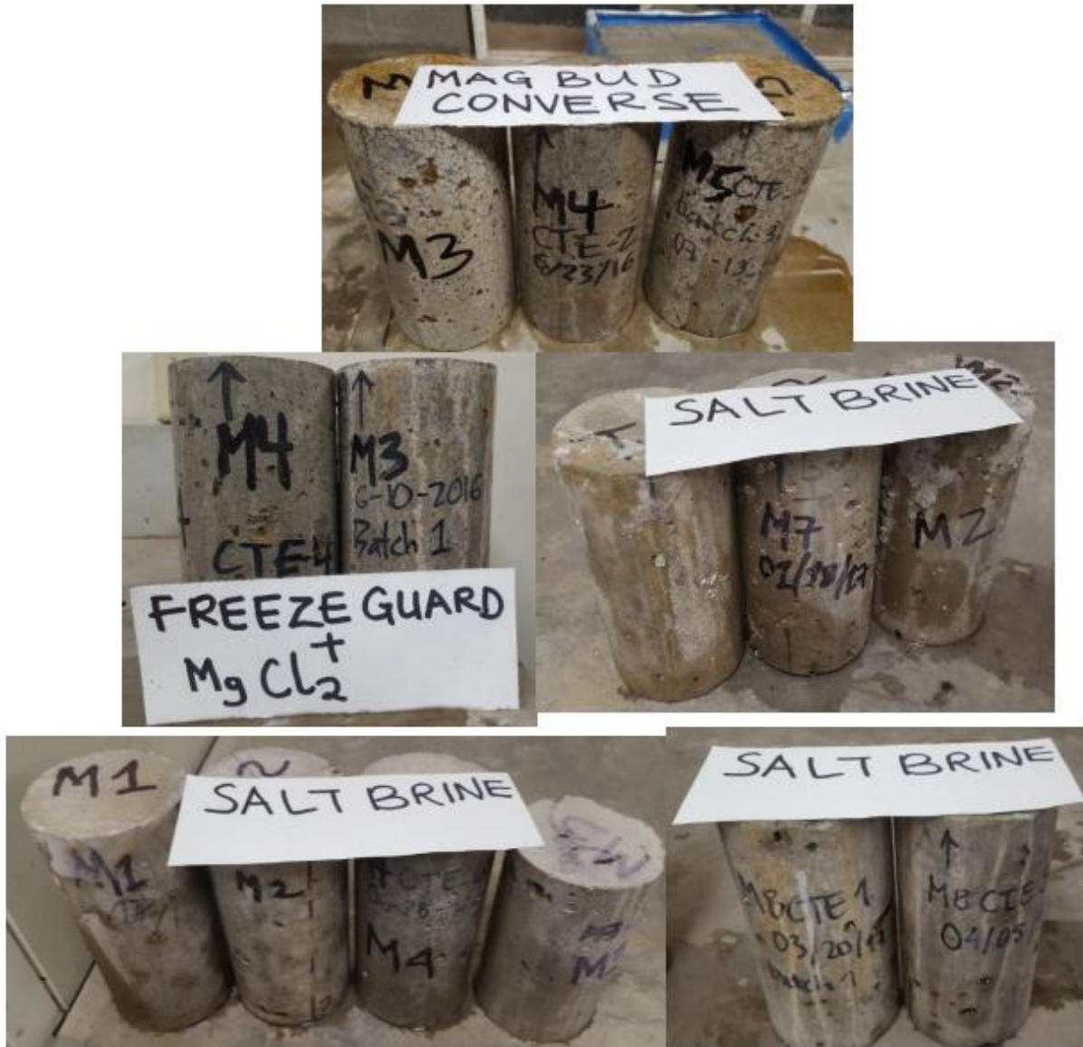
Figure 12. Concrete Specimens after 90 Days Continuous Soaking in Deicing Salt
