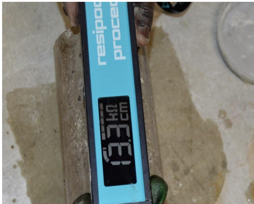
Figure 9. Surface Resistivity Testing
