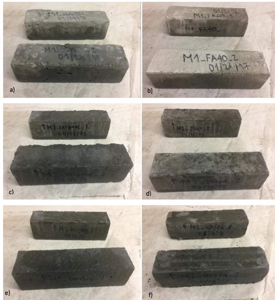
Figure 20. Results of F-T Cycles a) M1_ternary b) M1_FA40 c) M4_original d) M4_plain e) M4_ternary f) M4_FA40 g) M8_plain h) M8_ternary
