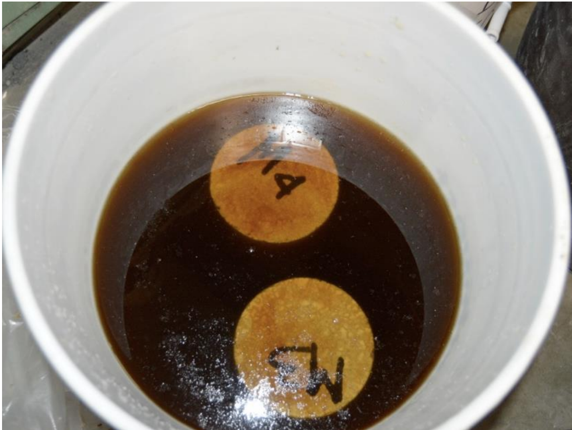
Figure 10. Concrete Specimens under Continuous Soaking
