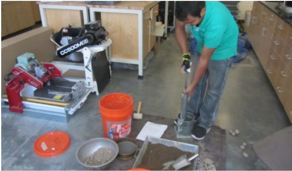
Figure 10. Subgrade Soil Specimen being Compacted for CBR Testing
