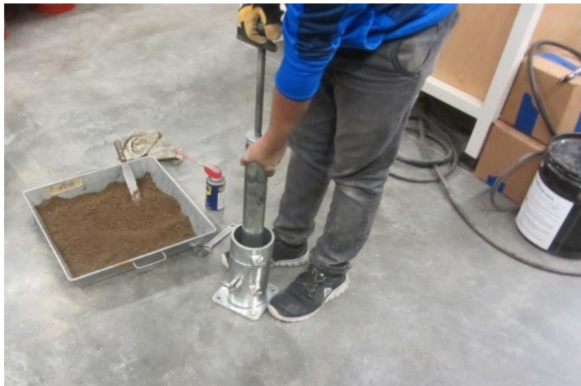
Figure 13. Photograph Showing Subgrade Specimen Preparation inside the Split Mold
