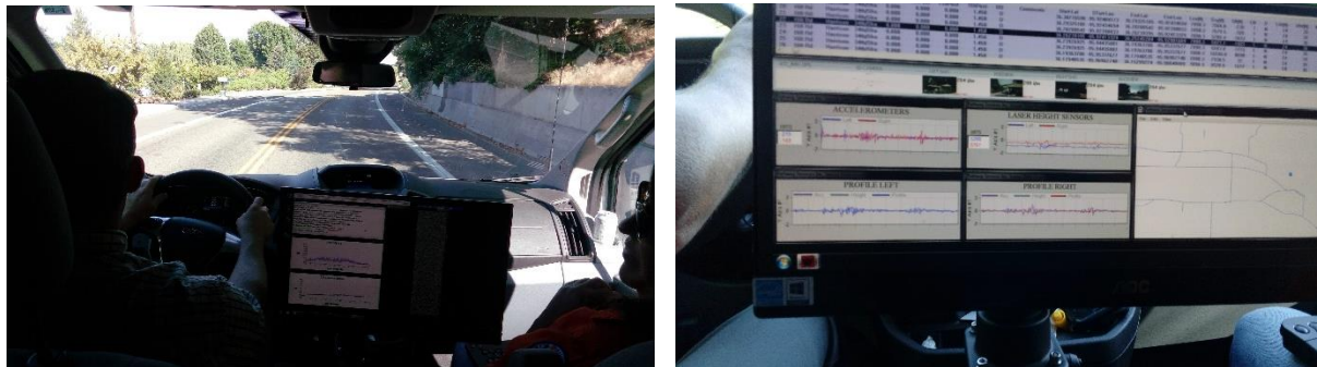
Figure 47. Photographs Showing the Workstation inside the Inertial Profiler Van
