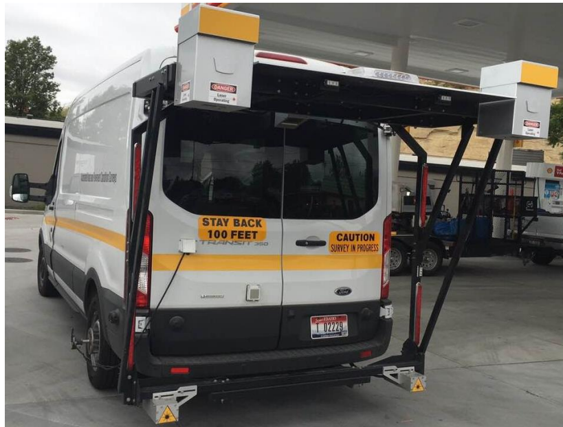
Figure 44. Photograph Showing ITD’s Inertial Profiler Van Used as a Reference Data Source in this Study
