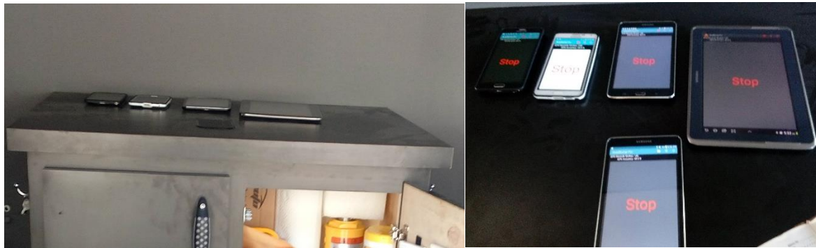
Figure 46. Photographs Showing Placement of the Mobile devices inside Inertial Profiler Van
