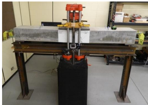
Figure 64. Typical three-point flexural beam test.
