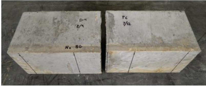
Figure 52. Interface bond test sample D-4 without bonding agent.
