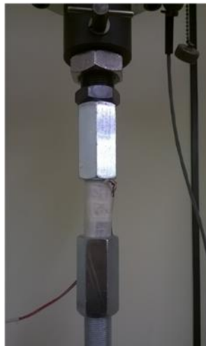
(a) Tension load cell used in headed bar pull-out tests
