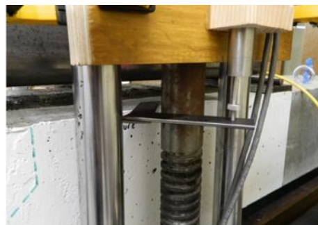
(b) LVDT mount and extension bracket
