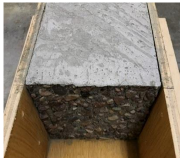
Figure 13. Exposed aggregate surface preparation.
