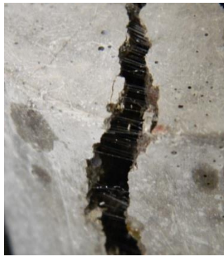
Figure 47. Split tensile crack showing the fibers.
