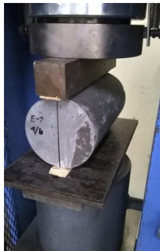
Figure 21. Splitting tensile testing setup.
