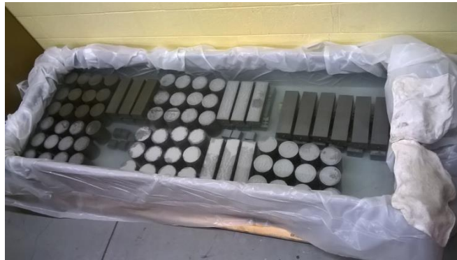
Figure 10. Water tank for moist curing of samples.
