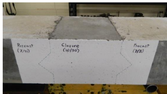
Figure 65. Beam specimen painted and interface lines drawn.
