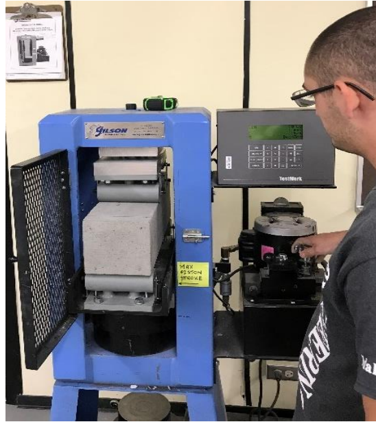
Figure 25. Interface bond test setup.
