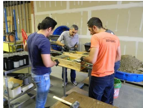
(b) Pouring rebar pull-out specimen precast segments
