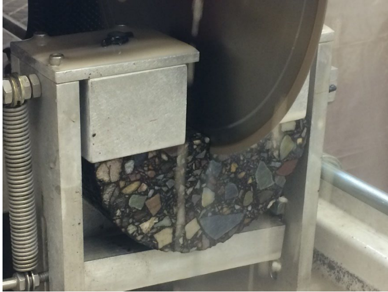
Figure 27: Photographs Showing: (a) Saw Cutting to Obtain the SCB Specimens; (b) Cutting the Notch into the SCB Puck
