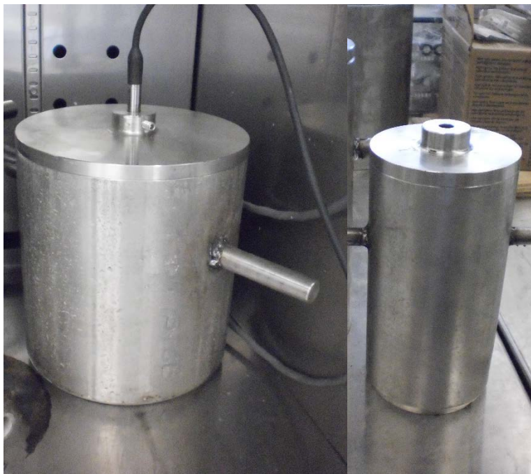
Figure 4.14. Two ACCT Setups Corresponding to Two Solution-to-Concrete Ratios: s/c = 3 (left) and s/c = 0.27 (right).
