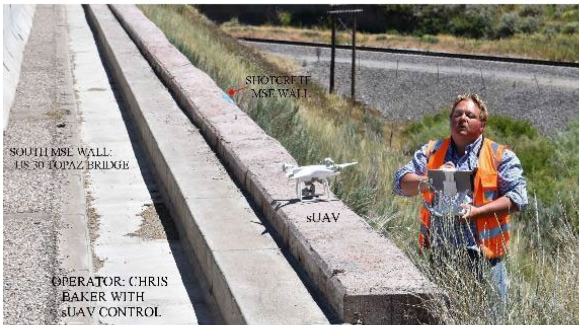
Figure 34. Photo of sUAV used in the ITD MSE Wall Investigation
