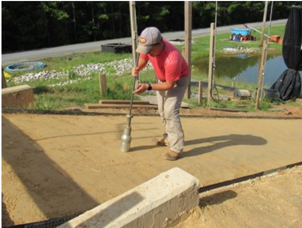
(a) Aligning cylinder with the slope
