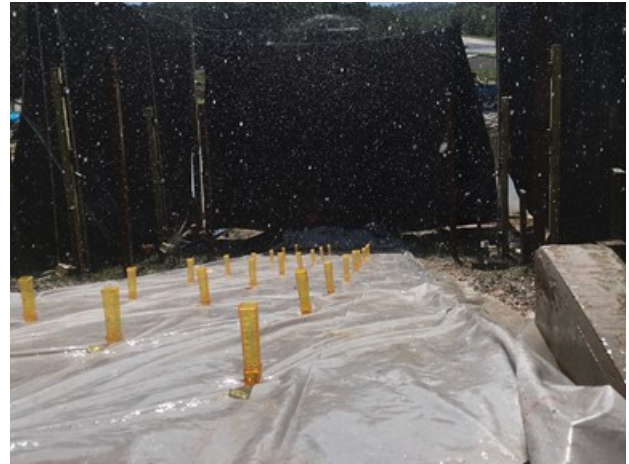
(b) Rainfall during calibration test
