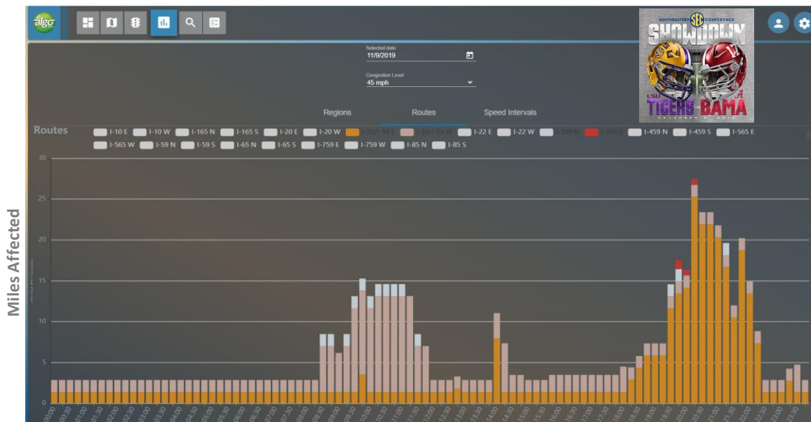
Figure 15 Traffic ticker (WCR only, grouped by freeway & direction, congestion threshold set at 45 mph)
