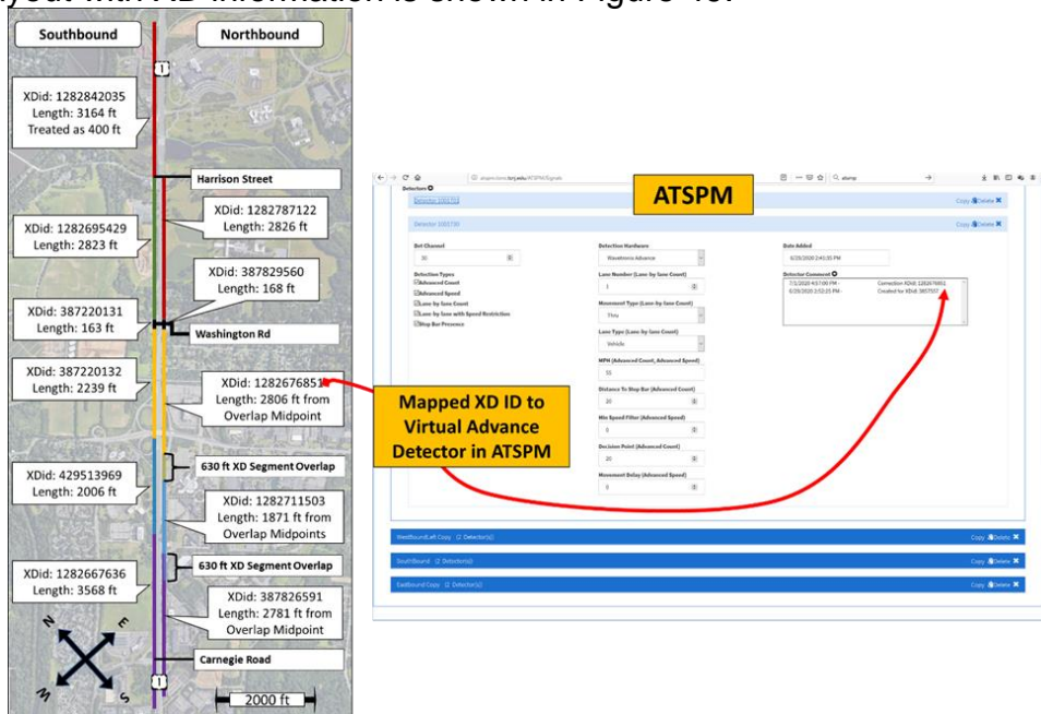
Figure 49. Virtual Advance Detector Layout (typical) for ATSPM Controllers
