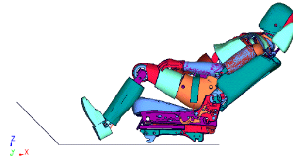
Figure 48. Rear-Impact Sled Test and FEA Simulation (45° Seat Back Angle)
